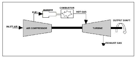
Figure 5 : A typical gas turbine unit
