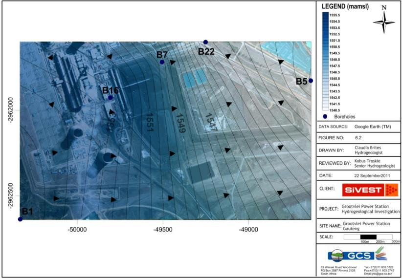
Figure 6-2: Groundwater Flow Directions
