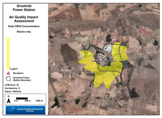
Figure 4-3: Highest predicted daily GLC for  $PM_{10}$  (stacks only after FFP retrofit at units 2, 3 and 4). Sensitive receptors shown on the plot are as follows: 1 – farm house; 2 – farm house; 3 – farm house; 4 - GVPS residential; 5 – farm house; 6 – farm house; 7 – farm house; 8 – Grootvlei.
