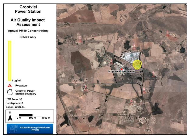
Figure 4-4: Annual predicted GLC for  $PM_{10}$  (stacks only after FFP retrofit at units 2, 3 and 4). Sensitive receptors shown on the plot are as follows: 1 – farm house; 2 – farm house; 3 – farm house; 4 - GVPS residential; 5 – farm house; 6 – farm house; 7 – farm house; 8 – Grootvlei.
