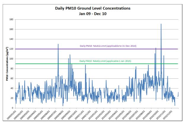
Figure 3-10: Daily measured  $PM_{10}$  ground level concentrations at Grootvlei for the period January 2009 to December 2010
