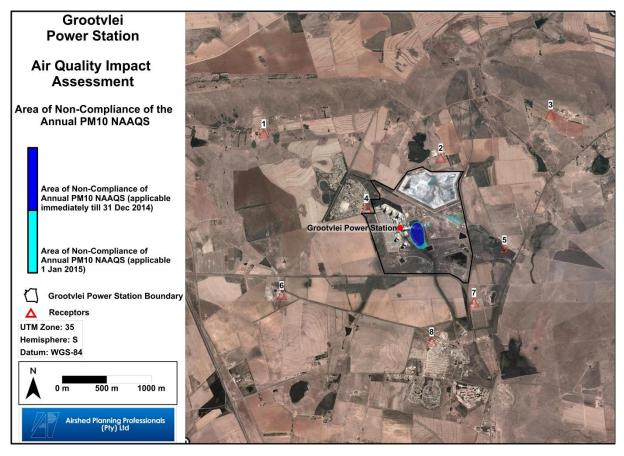
Figure 4-2: Annual predicted GLC for  $PM_{10}$  due to Grootvlei Power Station operations (after FFP retrofit at units 2, 3 and 4). Sensitive receptors shown on the plot are as follows: 1 – farm house; 2 – farm house; 3 – farm house; 4 - GVPS residential; 5 – farm house; 6 – farm house; 7 – farm house; 8 – Grootvlei.
