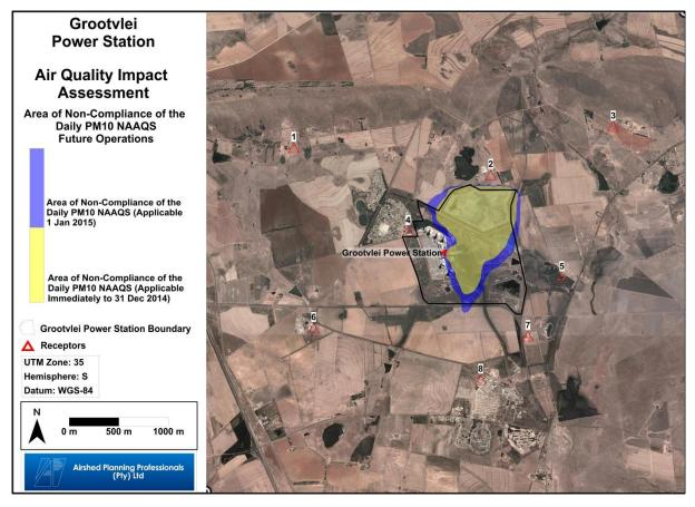
Figure 4-1: Area of exceedance of daily  $PM_{10}$  NAAQS due to Grootvlei Power Station operations (after FFP retrofit at units 2, 3 and 4). Sensitive receptors shown on the plot are as follows: 1 – farm house; 2 – farm house; 3 – farm house; 4 - GVPS residential; 5 – farm house; 6 – farm house; 7 – farm house; 8 – Grootvlei.
