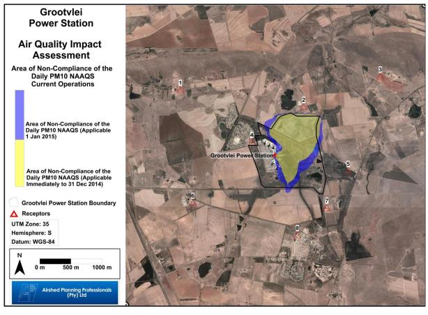
Figure 3-12: Area of exceedance of daily  $PM_{10}$  NAAQS due to current Grootvlei Power Station operations. Sensitive receptors shown on the plot are as follows: 1 – farm house; 2 – farm house; 3 – farm house; 4 - GVPS residential; 5 – farm house; 6 – farm house; 7 – farm house; 8 – Grootvlei.
