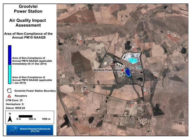
Figure 3-13: Annual predicted GLC for  $PM_{10}$  due to current Grootvlei Power Station operations. Sensitive receptors shown on the plot are as follows: 1 – farm house; 2 – farm house; 3 – farm house; 4 - GVPS residential; 5 – farm house; 6 – farm house; 7 – farm house; 8 – Grootvlei.
