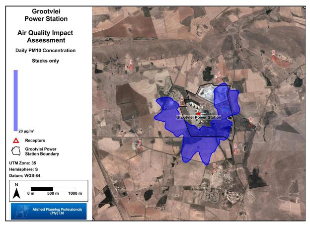
Figure 3-14: Highest predicted daily GLC for  $PM_{10}$  (stacks only). Sensitive receptors shown on the plot are as follows: 1 – farm house; 2 – farm house; 3 – farm house; 4 - GVPS residential; 5 – farm house; 6 – farm house; 7 – farm house; 8 – Grootvlei.
