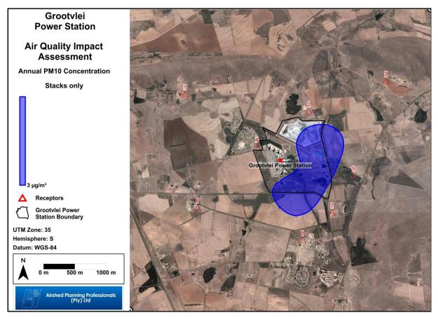
Figure 3-15: Annual predicted GLC for  $PM_{10}$  (stacks only). Sensitive receptors shown on the plot are as follows: 1 – farm house; 2 – farm house; 3 – farm house; 4 - GVPS residential; 5 – farm house; 6 – farm house; 7 – farm house; 8 – Grootvlei.
