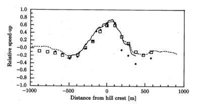
Figure 4.3: Relative speed-up ratios for flow over the Askervein hill at 10m above ground level. Measurements are indicated by dots and results from the orographic model by squares
