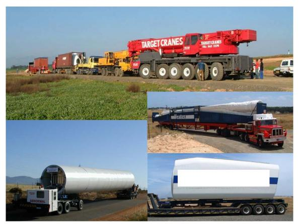
Figure 7.4: Photograph the illustrating equipment required for the transportation of turbine components to site (photographs courtesy of Eskom at during the construction of the Klipheuwel demonstration facility)
