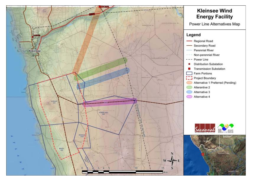
Figure 2: Map indicating proposed corridors for power line construction – alignments to be investigated in detail in the EIA Phase
