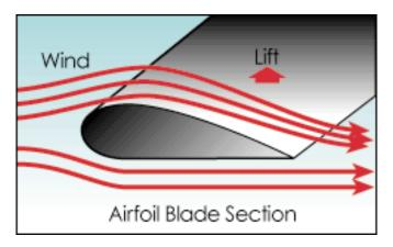
Figure 3.5: Illustration of the principle of lift
