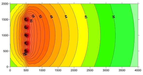
Figure 6-3: 5 WTGs operating, all hard ground scenario
