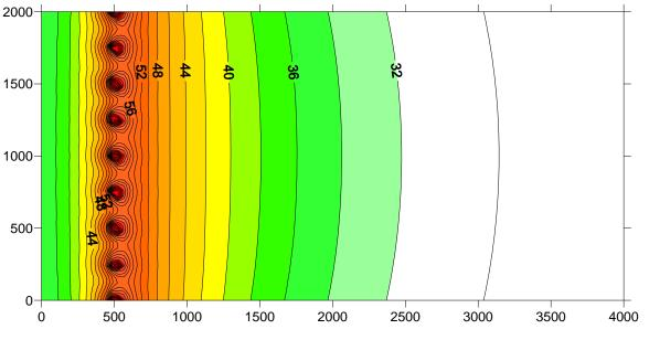
Figure 6-6: 13 WTGs operating. WTGs in one line on 500 m X-axes, all soft ground scenario
