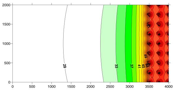
Figure 6-9: 52 WTGs operating in 4 lines (3500m, 3750m, 4000m and 4250m on X-axes) downwind from receptor, all hard ground scenario
