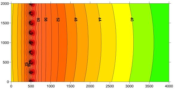
Figure 6-5: 13 WTGs operating, WTGs in one line on 500 m X-axes, all hard ground scenario
