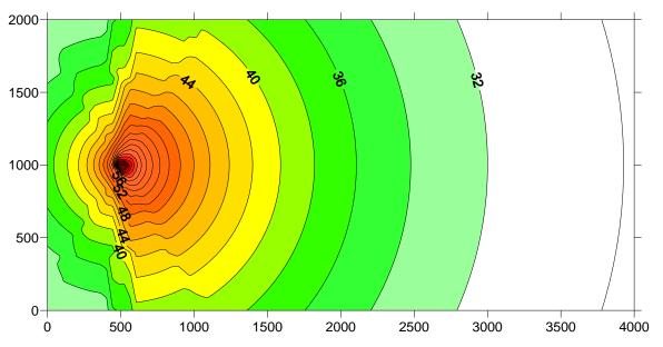
Figure 6-1: One WTG operating, all hard ground scenario
