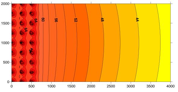
Figure 6-7: 52 WTGs operating in 4 lines (500, 250, 0, -250 on X-axes), all hard ground scenario
