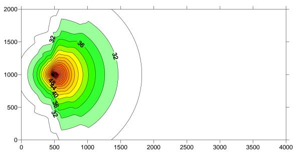
Figure 6-2: One WTG operating, all soft ground scenario (i.e vegetation attenuates some of the noise)
