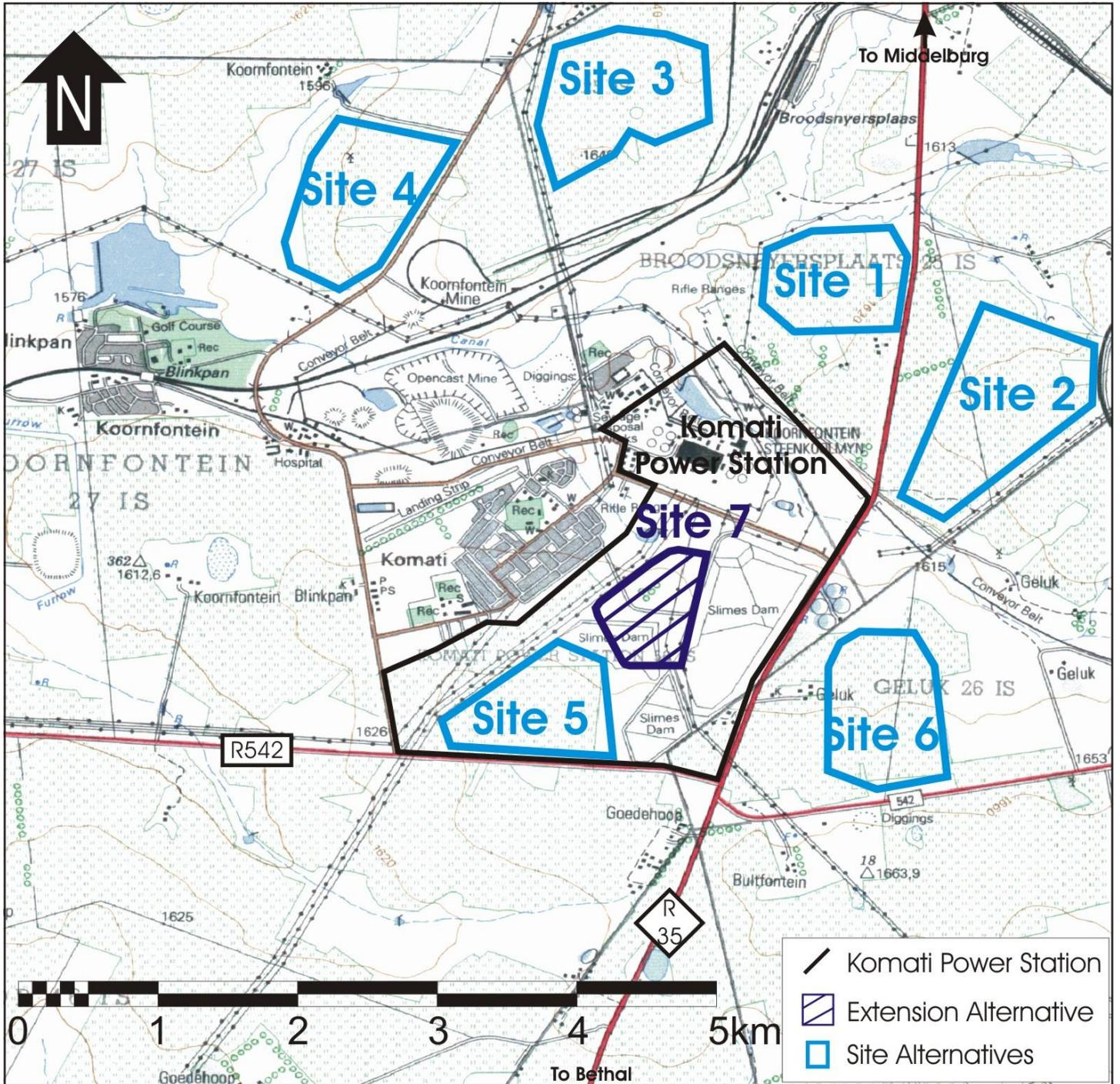
**Figure 2: Location of Site Alternatives for a New Ash Dam Facility at Komati Power Station**
