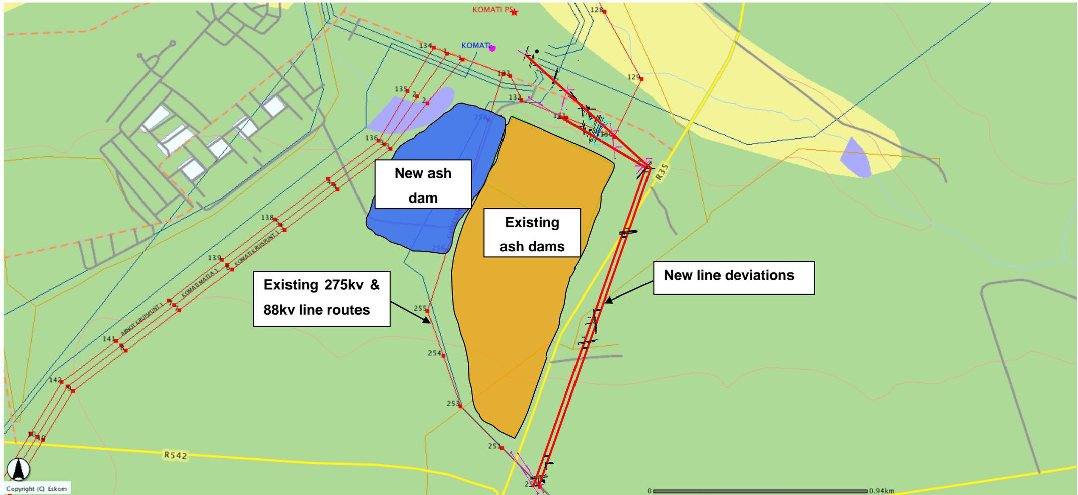
**Figure 10: Preferred Route for the Deviation of the 275 kv and 88kv Powerlines at Komati Power Station (TAP, 2007).**
