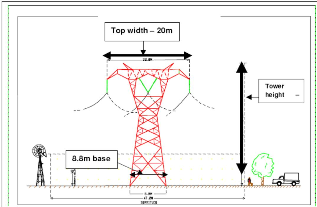
**Figure 11: Diagrammatic Representation of the Self-Supporting Strain Configuration Tower.**
