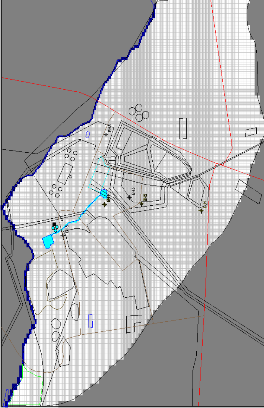
Figure 11. Komati Ash Dam numerical model grid.
