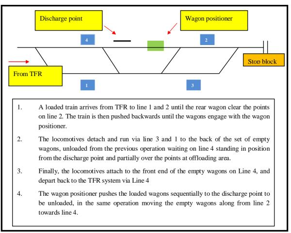
around the wagons on the loop to the opposite side of the unloading facility to pull clear the set of empty wagons unloaded during the previous operation, and the train will depart.
