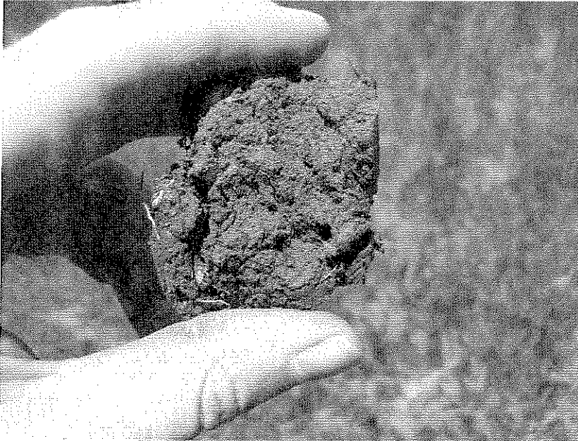
Example of soil and mottling from the seasonal zone in wetland Sehlakwane 1C.
