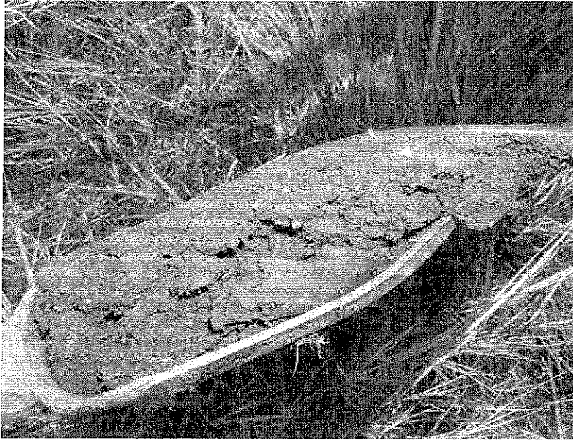
Soil sample taken at point LCV4. Note the clayey nature of the soil
