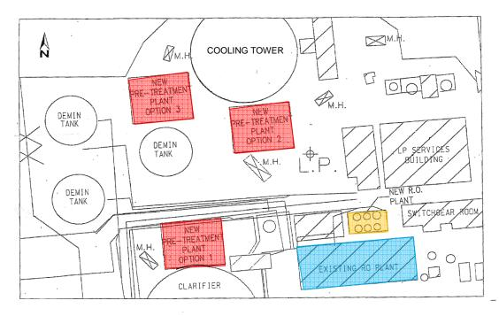
Figure 3.4 Alternative locations for the proposed pre-treatment plant (in red), the proposed RO/reject concentrator plant (in orange) and the existing RO (in blue)
