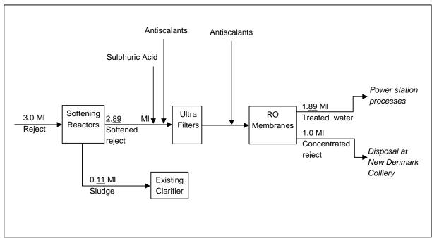
Figure 3.3 Process flow diagram of the proposed reject treatment plant (volume per day)
