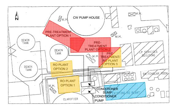
Figure 3.5 Alternative locations for the proposed pre-treatment plant (in red), the proposed RO/reject concentrator plant (in orange), proposed pipeline route corridors (dotted lines) and the existing RO (in blue)
