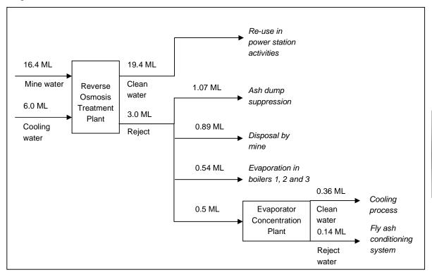
Figure 3.1 Process flow diagram of daily reject treatment and disposal
