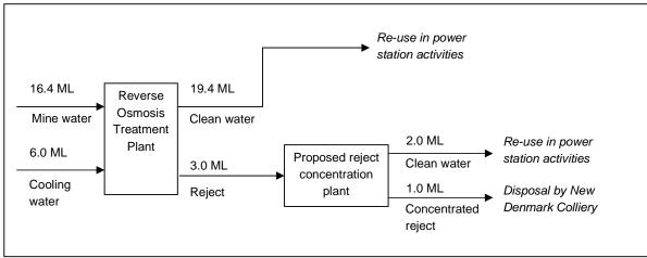
Figure 3.2 Process flow diagram of daily proposed reject treatment and disposal
