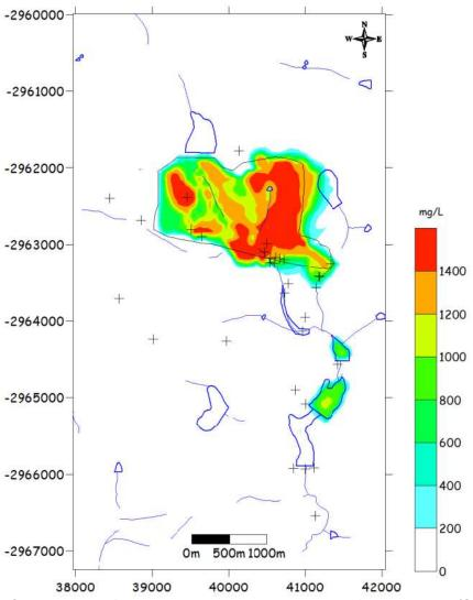
Figure 5.1 Current pollution plume extent, as modelled for sulphate (SO<sub>4</sub>) simulated concentrations
