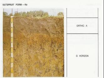
Figure 9-14: Katspruit Soil form (Soil Classification, 1991)
