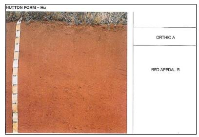
Figure 9-9: Hutton Soil Form (Soil Classification, 1991)
