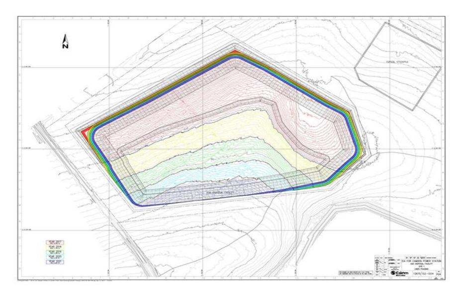
Figure 8-3: Lining requirements for the first five (5) years of ash disposal
