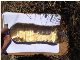
Figure 7: Excessive algal build-up
