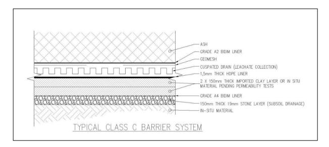
Figure 6-1: Class C Landfill Barrier System
