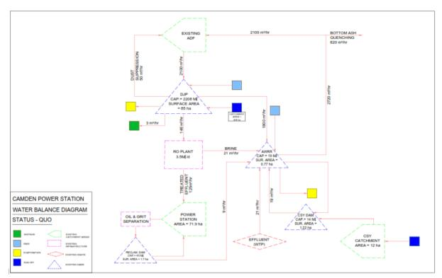
Figure 5-1: Stormwater System Diagram – Status Quo
