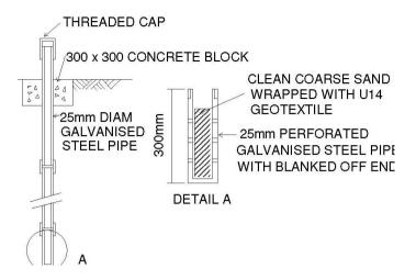
Figure 7-8: Typical piezometer detail
