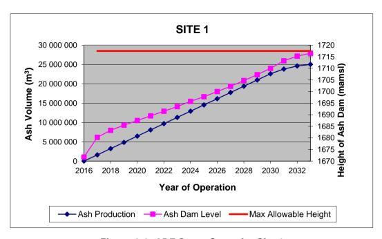
Figure 6-6: ADF Stage Curve for Site 1
