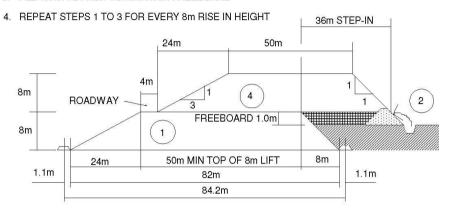
Figure 7-4: Day wall step-in process
