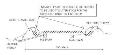
Figure 7-1: Construction of first ash berms
