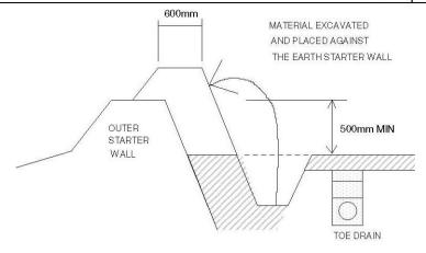
Figure 7-2: Construction of first berm and step
