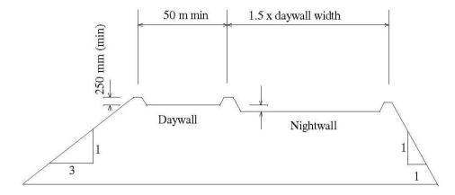
Figure 7-6: Day wall and nightfall construction
