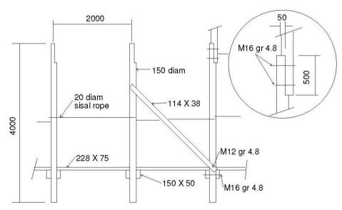
Figure 7-7: Typical walkway elevation
