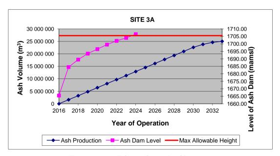
Figure 6-7: ADF Stage Curve for Site 3A
