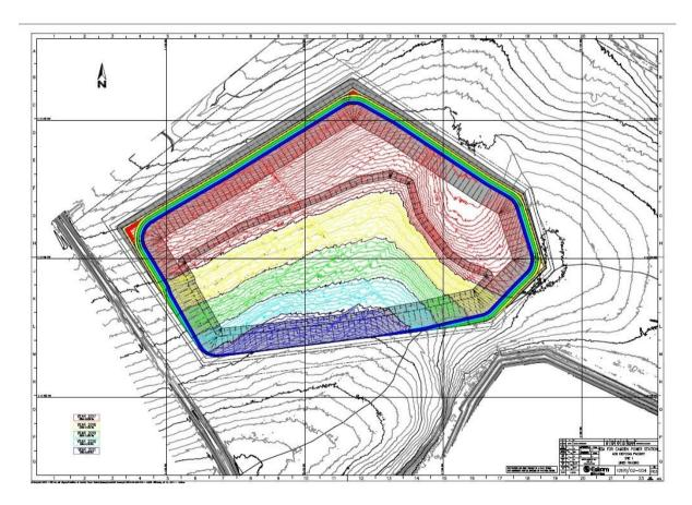
Figure 6-3: Lining requirements for the first five (5) years of ash disposal
