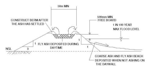
Figure 7-3: Wall building method
