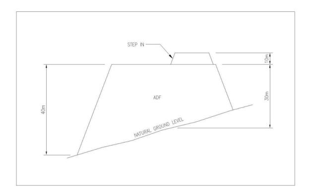
Figure 6-9: Sketch of Step-In and Height Restriction
