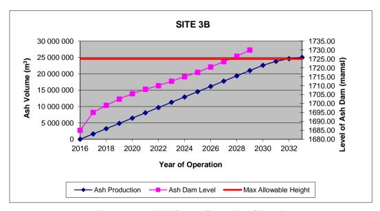
Figure 6-8: ADF Stage Curve for Site 3B
