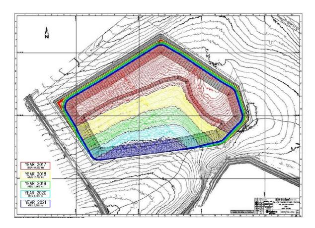
Figure 2-3: Lining requirements for the first five (5) years of ash disposal
