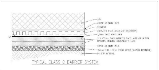
Figure 2-2: Proposed Class C landfill barrier system (DEA, 2011)
