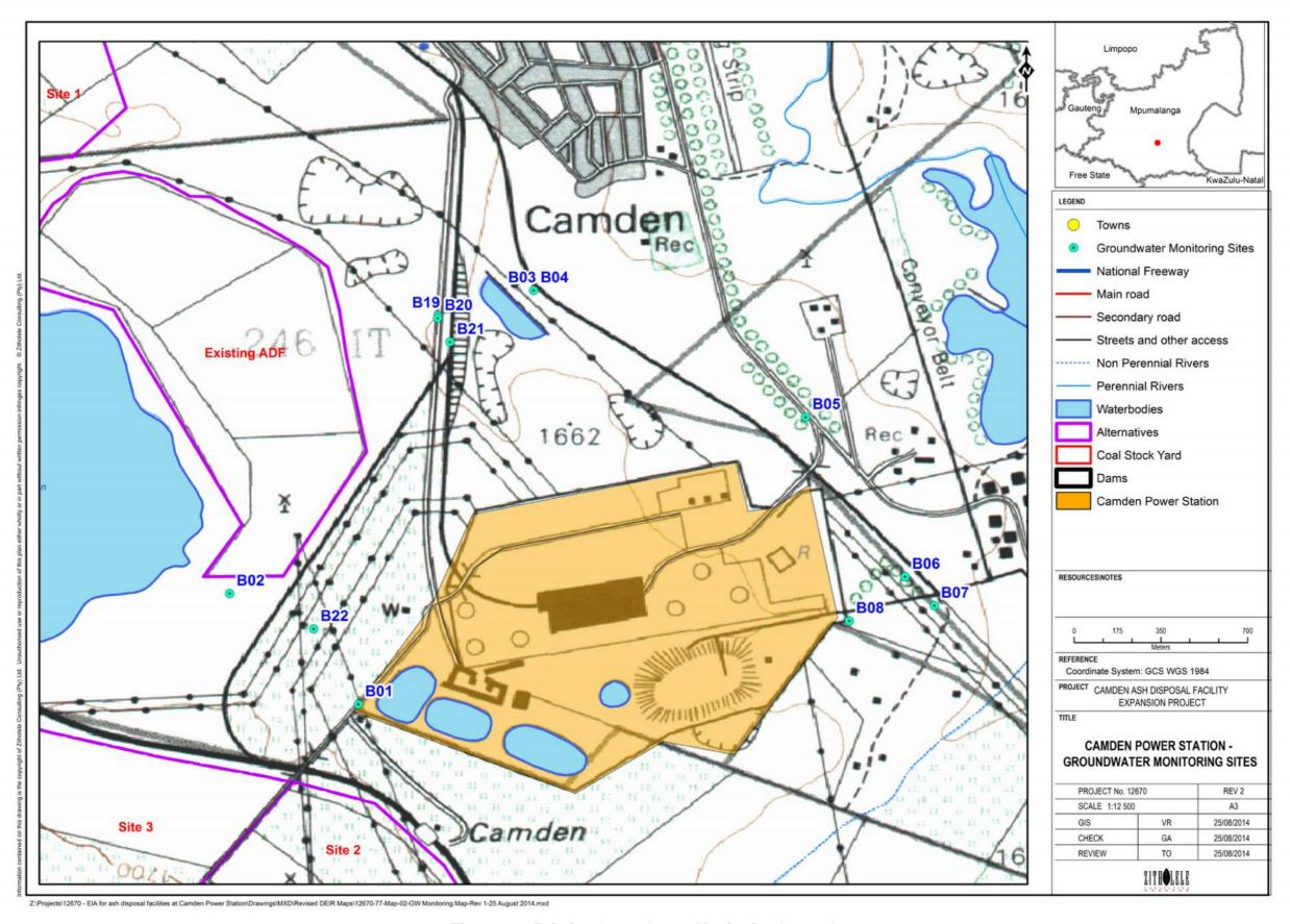
Figure 4-1: Existing Groundwater Monitoring Network
