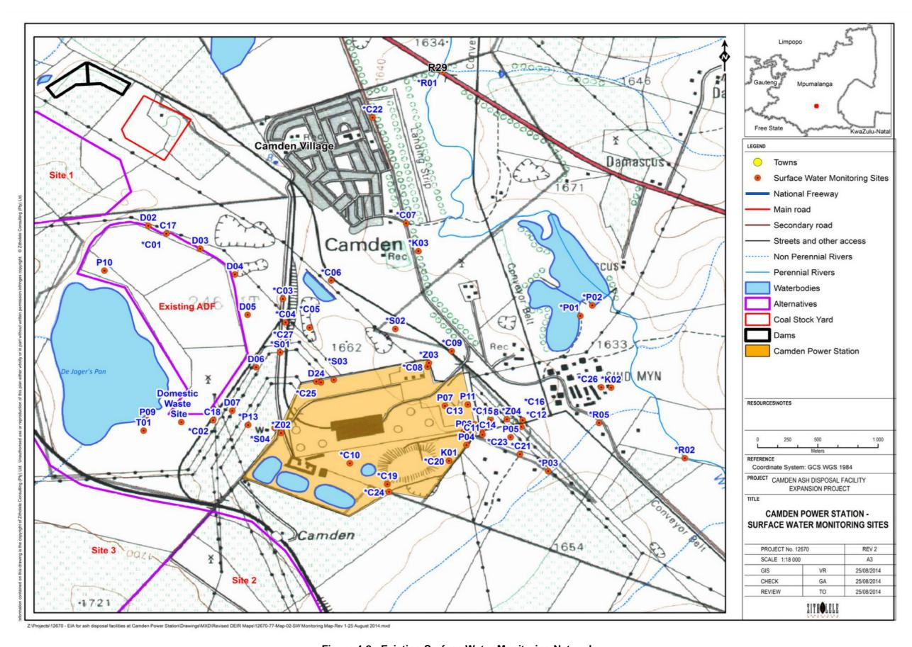
Figure 4-2 : Existing Surface Water Monitoring Network
