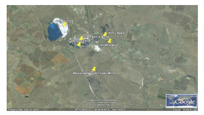
Figure 1. Camden Air / Quality Monitoring Station in relation to Camden Power Station and other pollution sources
