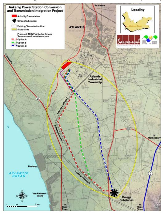
Figure 7.1: Transmission power line alternatives identified for investigation within the EIA process
