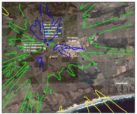
Figure A-85: Highest daily predicted NO<sub>2</sub> ground level concentrations (µg/m³) for the power station (NOx 600 µg/m³, 6 concentrations (µg/m³) for the power station (NOx 600 µg/m³, 6 units, operating 6 hours per day).
