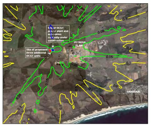
Figure A-61: Highest daily predicted  $SO_2$  ground level concentrations ( $\mu$ g/m³) for the power station (6 units, operating 6 hours per day).
