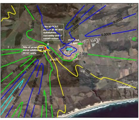
Figure A-20: Annual average predicted SO<sub>2</sub> ground level units at power station operating 2 hours per day).
