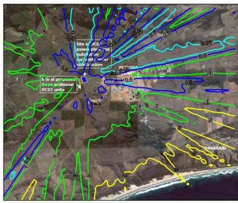
Figure A-18: Highest hourly predicted SO<sub>2</sub> ground level concentrations (µg/m³) for all sources (PetroSA refinery and 6 units at power station operating 2 hours per day).
