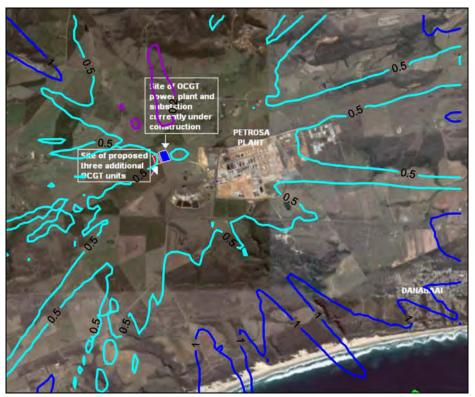
Figure A-73: Highest daily predicted NO<sub>2</sub> ground level Figure A-74: concentrations (µg/m³) for the power station (NOx 165 µg/m³, 6 concentrations (µg/m³) for the power station (NOx 165 µg/m³, 6 units, operating 6 hours per day).
