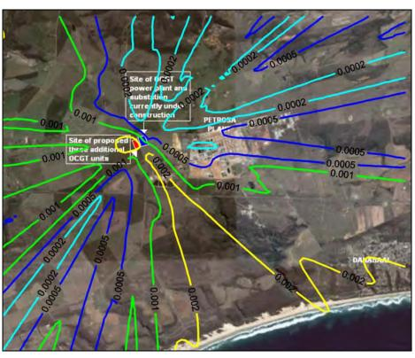
Figure A-14: Annual average predicted  $SO_2$  ground level concentrations ( $\mu g/m^3$ ) for the power station (6 units, operating 2 hours per day).
