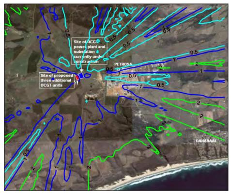
Highest daily predicted NO<sub>2</sub> ground level Figure A-38: Figure A-37: concentrations (µg/m³) for the power station (NOx 600 µg/m³, 6 concentrations (µg/m³) for the power station (NOx 600 µg/m³, 6 units, operating 2 hours per day).
