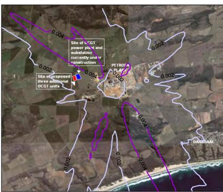
Figure A-64: Highest daily predicted  $SO_2$  ground level concentrations ( $\mu g/m^3$ ) for the PetroSA refinery.
