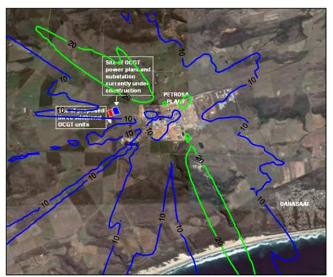
Figure A-43: Highest daily predicted NO<sub>2</sub> ground level Figure A-44: concentrations (µg/m³) for all sources (PetroSA refinery and 6 concentrations (µg/m³) for all sources (PetroSA refinery and 6 units at power station operating 2 hours per day).
