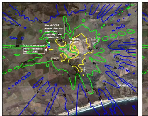
Figure A-47: Highest hourly predicted CO ground level Figure A-48: concentrations (µg/m³) for the PetroSA refinery.
