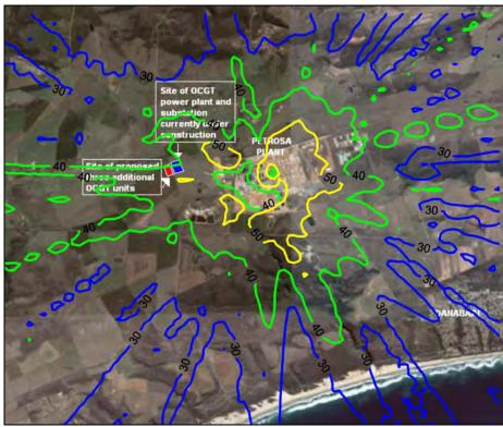
Figure A-96: Highest hourly predicted CO ground level concentrations (µg/m³) for all sources (PetroSA refinery and 6 units at power station operating 6 hours per day).
