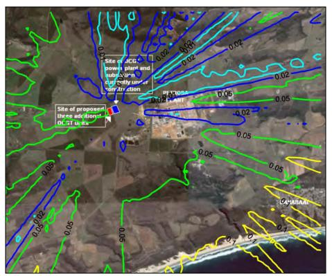
Highest daily predicted SO<sub>2</sub> ground level Figure A-19: concentrations (µg/m³) for all sources (PetroSA refinery and 6 concentrations (µg/m³) for all sources (PetroSA refinery and 6 units at power station operating 2 hours per day).
