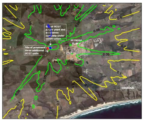
Highest daily predicted SO<sub>2</sub> ground level Figure A-68: Figure A-67: concentrations (µg/m³) for all sources (PetroSA refinery and 6 concentrations (µg/m³) for all sources (PetroSA refinery and 6 units at power station operating 6 hours per day).
