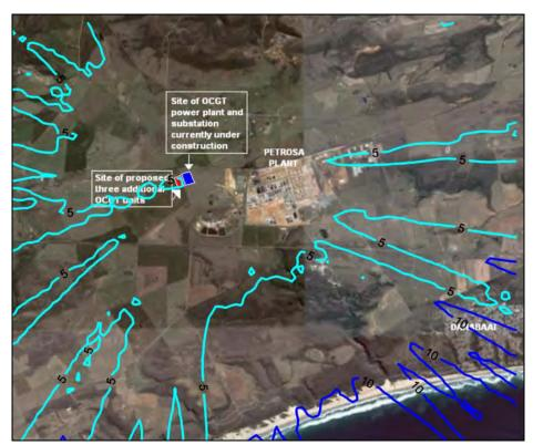
Highest hourly predicted NO<sub>2</sub> ground level Figure A-22: Figure A-21: concentrations (µg/m³) for the power station (NOx 165 µg/m³, 3 concentrations (µg/m³) for the power station (NOx 165 µg/m³, 3 units, operating 2 hours per day).
