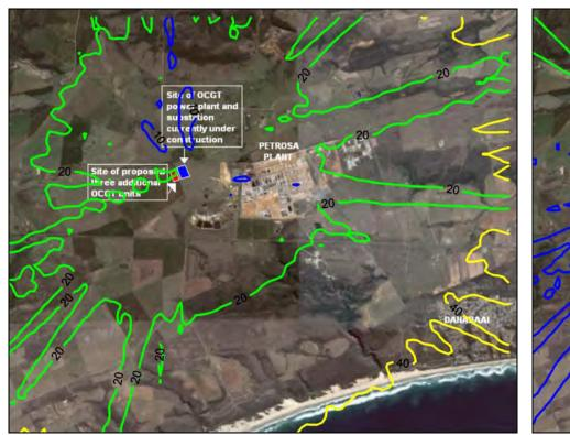
Highest hourly predicted NO<sub>2</sub> ground level Figure A-82: Figure A-81: concentrations (µg/m³) for the power station (NOx 600 µg/m³, 3 concentrations (µg/m³) for the power station (NOx 600 µg/m³, 3 units, operating 6 hours per day).
