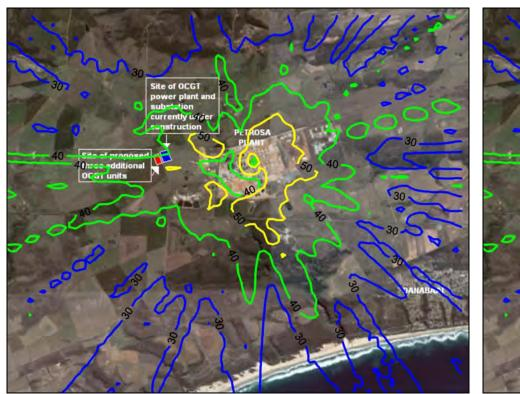
Figure A-95: Highest hourly predicted CO ground level Figure A-96: concentrations (µg/m³) for the PetroSA refinery.
