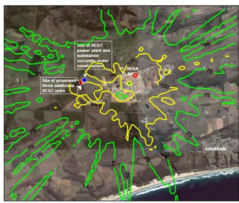
Figure A-30: Highest hourly predicted NO<sub>2</sub> ground level concentrations (μg/m³) for all sources (PetroSA refinery and 6 units at power station operating 2 hours per day).
