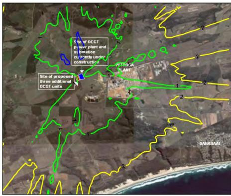
Figure A-66: Highest hourly predicted  $SO_2$  ground level concentrations ( $\mu g/m^3$ ) for all sources (PetroSA refinery and 6 units at power station operating 6 hours per day).
