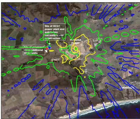
Figure A-48: Highest hourly predicted CO ground level concentrations (µg/m³) for all sources (PetroSA refinery and 6 units at power station operating 2 hours per day).
