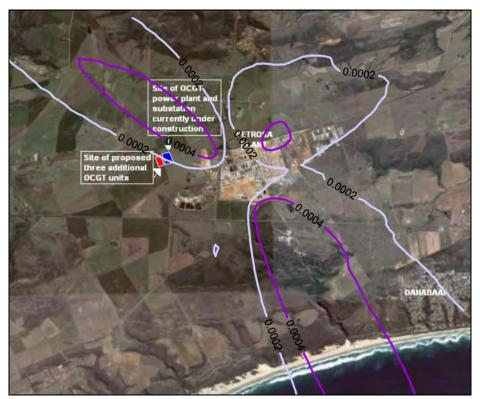
Figure A-65: Annual average predicted SO<sub>2</sub> ground level Figure A-66: concentrations (µg/m³) for the PetroSA refinery.
