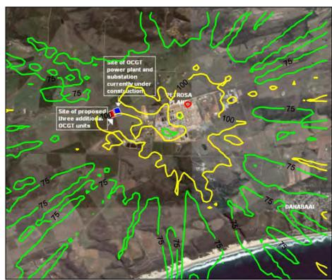
Figure A-42: Highest hourly predicted  $NO_2$  ground level concentrations ( $\mu g/m^3$ ) for all sources (PetroSA refinery and 6 units at power station operating 2 hours per day).
