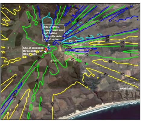
Figure A-36: Highest hourly predicted  $NO_2$  ground level concentrations ( $\mu$ g/m³) for the power station ( $NOx~600~\mu$ g/m³, 6 units, operating 2 hours per day).
