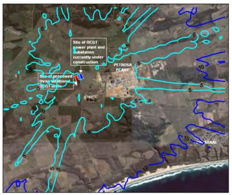
Highest hourly predicted NO<sub>2</sub> ground level Figure A-70: Figure A-69: concentrations (µg/m³) for the power station (NOx 165 µg/m³, 3 concentrations (µg/m³) for the power station (NOx 165 µg/m³, 3 units, operating 6 hours per day).
