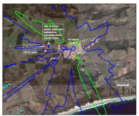
Figure A-31: Highest daily predicted NO<sub>2</sub> ground level Figure A-32: concentrations (µg/m³) for all sources (PetroSA refinery and 6 concentrations (µg/m³) for all sources (PetroSA refinery and 6 units at power station operating 2 hours per day).
