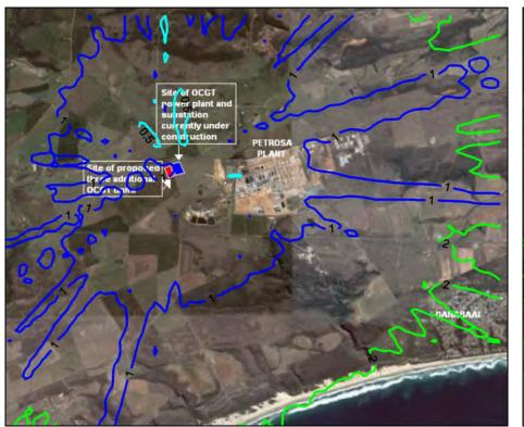
Figure A-93: Highest hourly predicted CO ground level Figure A-94: concentrations (µg/m³) for the power station (3 units, operating 6 concentrations hours per day).
