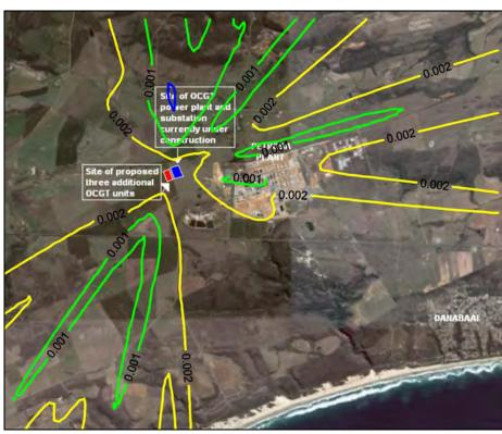
Figure A-62: Annual average predicted  $SO_2$  ground level concentrations ( $\mu g/m^3$ ) for the power station (6 units, operating 6 hours per day).
