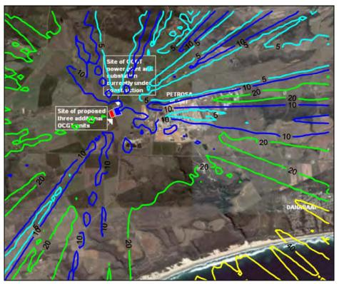
Highest hourly predicted NO<sub>2</sub> ground level Figure A-34: Figure A-33: concentrations (µg/m³) for the power station (NOx 600 µg/m³, 3 concentrations (µg/m³) for the power station (NOx 600 µg/m³, 3 units, operating 2 hours per day).
