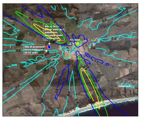
Figure A-55: Highest daily predicted PM10 ground level Figure A-56: concentrations (µg/m³) for all sources (PetroSA refinery and 6 concentrations (µg/m³) for all sources (PetroSA refinery and 6 units at power station operating 6 hours per day).
