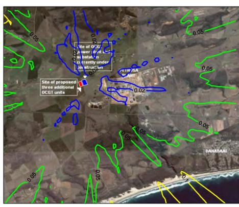
Figure A-58: Highest daily predicted  $SO_2$  ground level concentrations ( $\mu g/m^3$ ) for the power station (3 units, operating 6 hours per day).
