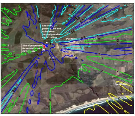
Figure A-46: Highest hourly predicted CO ground level concentrations ( $\mu$ g/m³) for the power station (6 units, operating 2 hours per day).
