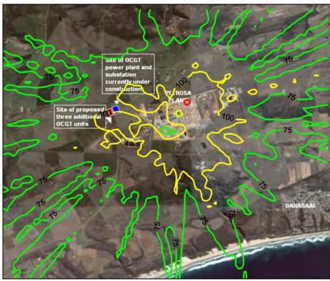
Figure A-78: Highest hourly predicted NO<sub>2</sub> ground level concentrations (μg/m³) for all sources (PetroSA refinery and 6 units at power station operating 6 hours per day).
