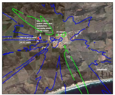
Highest daily predicted NO<sub>2</sub> ground level Figure A-92: Figure A-91: concentrations (µg/m³) for all sources (PetroSA refinery and 6 concentrations (µg/m³) for all sources (PetroSA refinery and 6 units at power station operating 6 hours per day).
