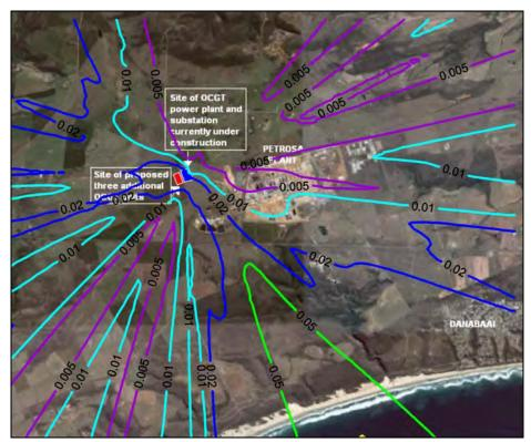
Figure A-35: Annual average predicted  $NO_2$  ground level concentrations ( $\mu g/m^3$ ) for the power station (NOx 600  $\mu g/m^3$ , 3 units, operating 2 hours per day).
