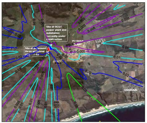
Annual average predicted NO<sub>2</sub> ground level Figure A-84: Figure A-83: concentrations (µg/m³) for the power station (NOx 600 µg/m³, 3 concentrations (µg/m³) for the power station (NOx 600 µg/m³, 6 units, operating 6 hours per day).
