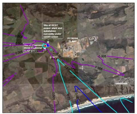
Figure A-23: Annual average predicted NO<sub>2</sub> ground level concentrations (µg/m³) for the power station (NOx 165 µg/m³, 3 concentrations (µg/m³) for the power station (NOx 165 µg/m³, 6 units, operating 2 hours per day).
