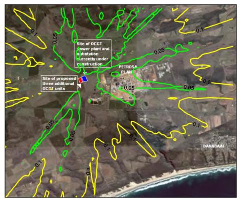
Figure A-49: Highest daily predicted PM10 ground level Figure A-50: concentrations (µg/m³) for the power station (3 units, operating 6 concentrations (µg/m³) for the power station (3 units, operating 6 hours per day).
