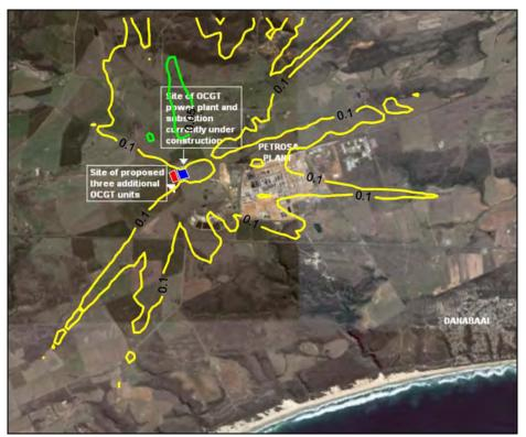
Figure A-51: Highest daily predicted PM10 ground level Figure A-52: concentrations (µg/m³) for the power station (6 units, operating 6 concentrations (µg/m³) for the power station (6 units, operating 6 hours per day).
