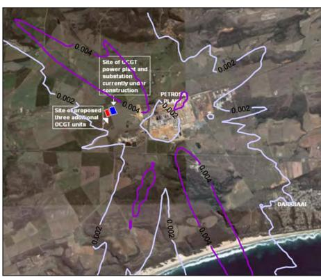
Figure A-16: Highest daily predicted  $SO_2$  ground level concentrations ( $\mu g/m^3$ ) for the PetroSA refinery.
