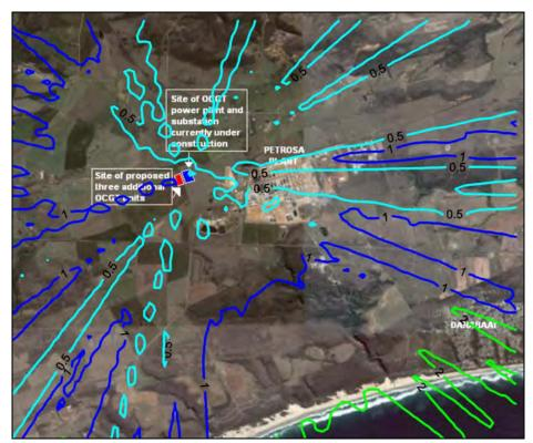
Figure A-45: Highest hourly predicted CO ground level concentrations ( $\mu g/m^3$ ) for the power station (3 units, operating 2 hours per day).
