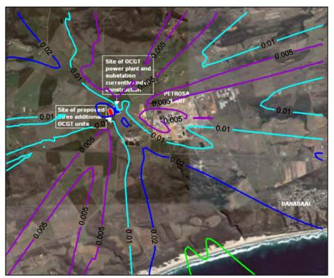
Figure A-71: Annual average predicted NO<sub>2</sub> ground level Figure A-72: concentrations (µg/m³) for the power station (NOx 165 µg/m³, 3 concentrations (µg/m³) for the power station (NOx 165 µg/m³, 6 units, operating 6 hours per day).
