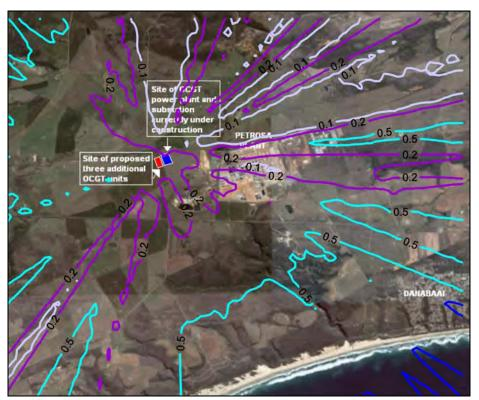
Figure A-25: Highest daily predicted NO<sub>2</sub> ground level Figure A-26: concentrations (µg/m³) for the power station (NOx 165 µg/m³, 6 concentrations (µg/m³) for the power station (NOx 165 µg/m³, 6 units, operating 2 hours per day).
