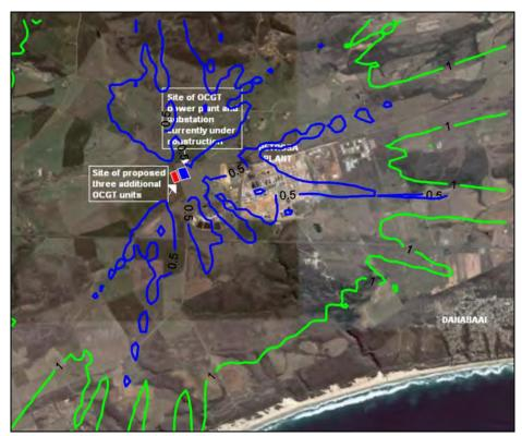
Figure A-57: Highest hourly predicted  $SO_2$  ground level Figure A-58: concentrations ( $\mu$ g/m³) for the power station (3 units, operating 6 hours per day).
