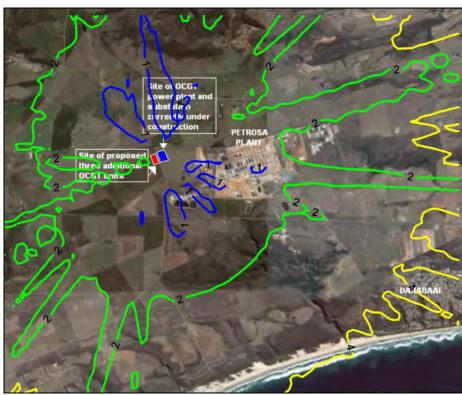
Figure A-94: Highest hourly predicted CO ground level concentrations ( $\mu$ g/m³) for the power station (6 units, operating 6 hours per day).
