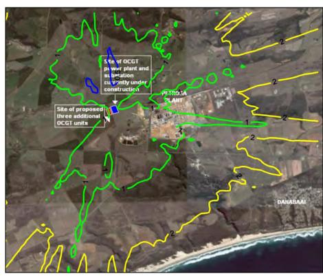
Figure A-60: Highest hourly predicted  $SO_2$  ground level concentrations ( $\mu$ g/m³) for the power station (6 units, operating 6 hours per day).
