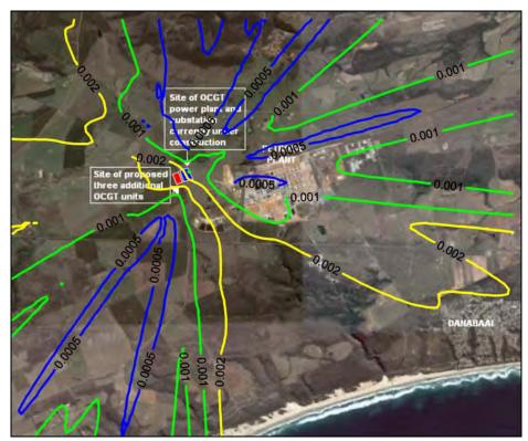
Figure A-59: Annual average predicted  $SO_2$  ground level Figure A-60: concentrations ( $\mu$ g/m³) for the power station (3 units, operating 6 concentration hours per day).
