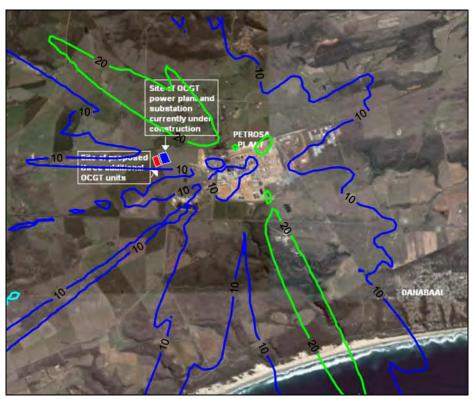
Figure A-79: Highest daily predicted NO<sub>2</sub> ground level Figure A-80: concentrations (µg/m³) for all sources (PetroSA refinery and 6 concentrations (µg/m³) for all sources (PetroSA refinery and 6 units at power station operating 6 hours per day).
