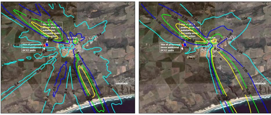
Figure A-53: Highest daily predicted PM10 ground level Figure A-54: concentrations ( $\mu g/m^3$ ) for the PetroSA refinery.
