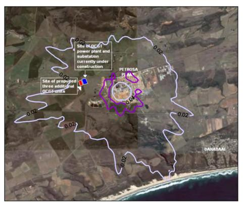
Figure A-15: Highest hourly predicted SO<sub>2</sub> ground level Figure A-16: concentrations (µg/m³) for the PetroSA refinery.
