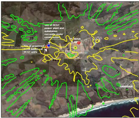
Figure A-90: Highest hourly predicted NO<sub>2</sub> ground level concentrations (μg/m³) for all sources (PetroSA refinery and 6 units at power station operating 6 hours per day).
