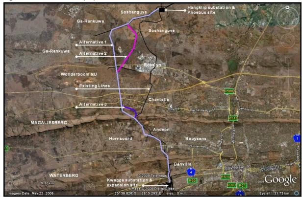
Figure 3: Overview of the proposed 400kV Transmission Power Line Route Alternatives
