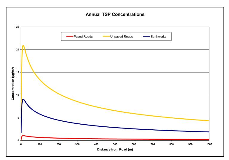
Figure 4-2: Annual average TSP concentrations due to vehicle entrainment on paved and unpaved road surfaces as well as earthworks for proposed construction operations.
