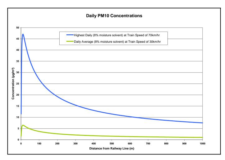
Figure 4-7: Daily PM10 concentrations due to wind-blown sorbent material from moving rail carts during operational activities.
