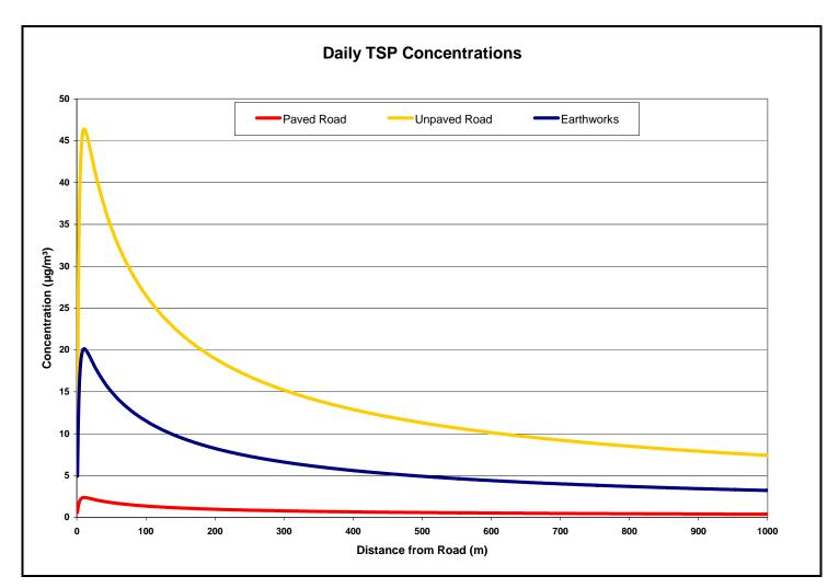
Figure 4-1: Daily TSP concentrations due to vehicle entrainment on paved and unpaved road surfaces as well as earthworks for proposed construction operations.
