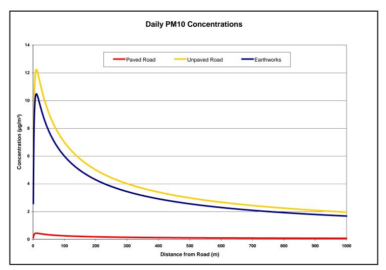
Figure 4-3: Daily PM10 concentrations due to vehicle entrainment on paved and unpaved road surfaces as well as earthworks for proposed construction operations.
