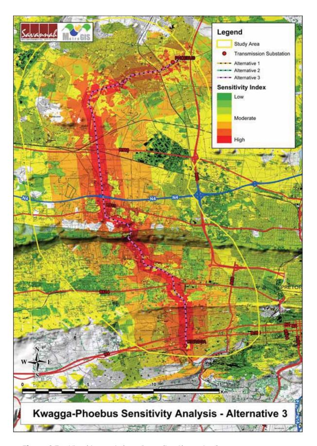
**Figure 6.5:** Visual impact index – Power line Alternative 3
