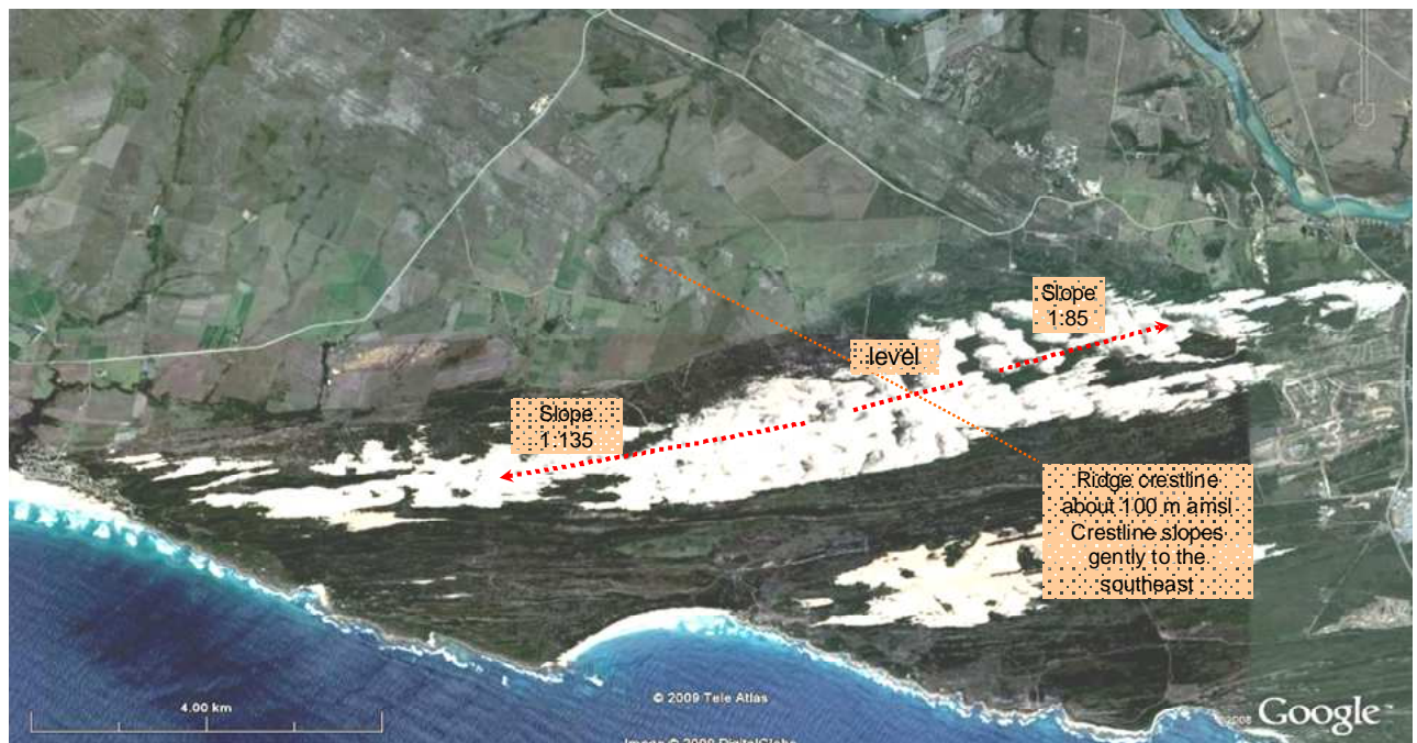
Figure 2.19. Slopes of the interdune surfaces in the Oyster Bay dunefield. The slope is steeper in the eastern sector of the dunefield. Base photo is the Google image of 2004.
