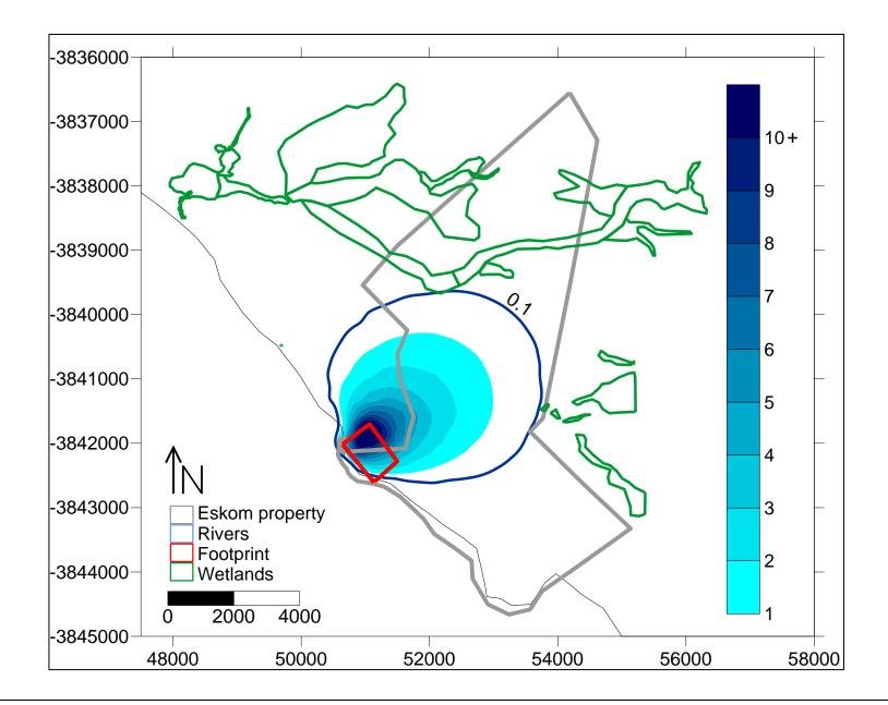
Figure 4.3 Modelled radius of drawdown at the Bantamsklip site. Figure after Visser *et al* (2011). Drawdown model based on dewatering of an area equivalent to one third of one NPS footprint.
