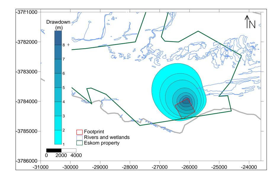
Figure 4.7 Modelled radius of drawdown at the Thyspunt site, assuming draw-down of eastern half of proposed NPS footprint. Figure after Visser et al. (2011). Note that the extent of coastal seeps is not clear at this scale, and Figure 2.6 should be referred to, for a clearer indication of coastal seep extent. Wetlands shown in blue.
