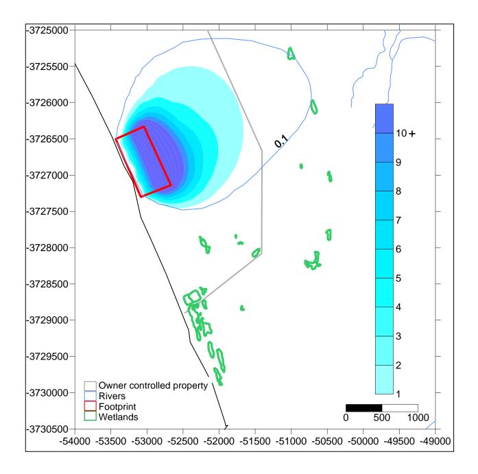
Figure 4.1C Modelled sensitivity of wetlands on the Duynefontein site to construction-associated groundwater drawdown. Model based on drawdown of the entire NPS footprint, and thus an exaggeration of extent of impact. Figure after Visser et al. (2011).
