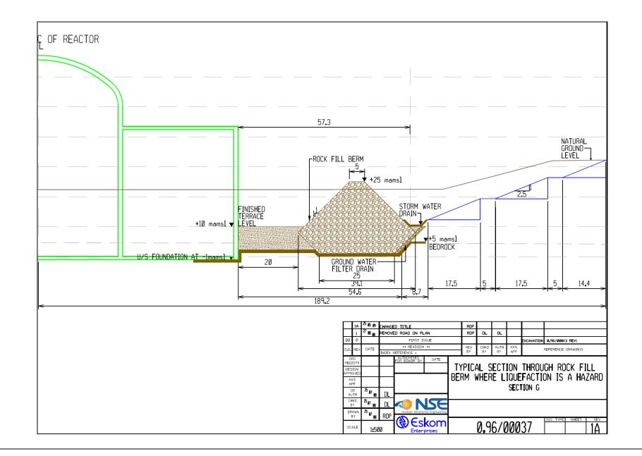
Figure 3.5 Proposed approach to stabilisation of potential liquefaction areas at the Thyspunt site, showing stormwater drain. Figure courtesy Eskom. Conceptual diagram only – may change in final design.
