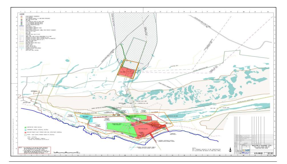
Figure 3.3 Thyspunt site, showing the areas proposed for the location of different components of the NPS and its ancillary structures, as well as conceptual footprints for the terrace of a 4000 MW plant, a topsoil stockpile and a spoil stockpile. Figure courtesy Eskom.
