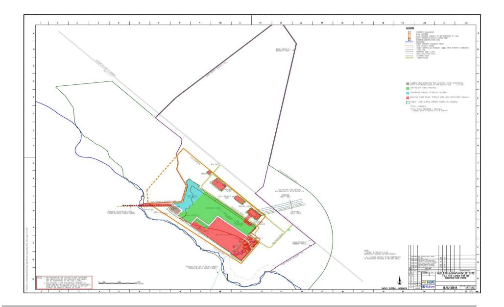
Figure 3.2 Bantamsklip site, showing the areas proposed for the location of different components of the NPS and its ancillary structures, as well as conceptual footprints for the terrace of a 4000 MW plant, a topsoil stockpile and a spoil stockpile. Figure courtesy Eskom.
