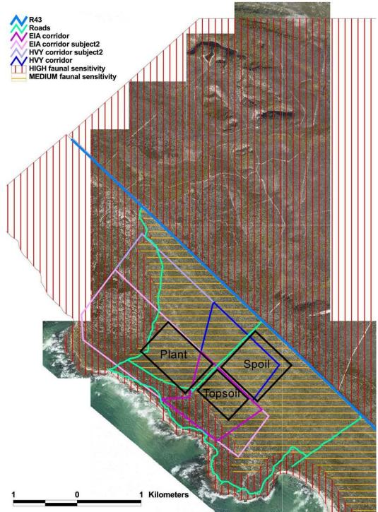
**Figure 48:** Recommended footprints for the Bantamsklip site. The plant, topsoil and spoil footprints are to the scale provided by Eskom. Note that the recommended footprint avoids the dunes to the northwest and limestone ridge to the southeast, and makes provision for a broad coastal corridor.
