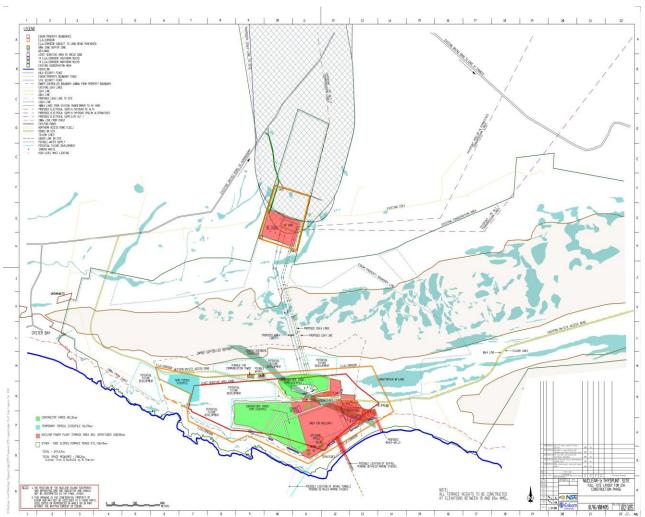
Figure 45: Site boundaries and development corridor, and associated infrastructure at Thyspunt. Note that the HV yard is situated on the inland portion, some distance from the development corridor for the plant.
