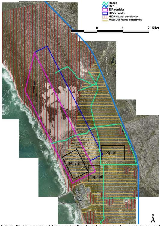
**Figure 46:** Recommended footprints for the Duynefontein site. The plant, topsoil and spoil footprints are to the scale provided by Eskom. Note that the recommended footprints avoid the mobile dunes to the north, and make provision for a wide coastal corridor and a corridor between KNPS and the Nuclear-1 NPS.
