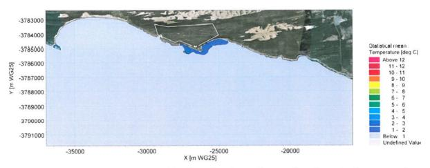
**Figure 5:** Mean temperature increase arising from the release of warmed cooling water from a nearshore piped outlet (extracted from the presentation to the Squid Scientific Working Group by the independent marine consultants)
