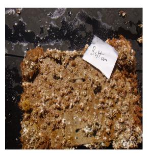
Plate deployed 8 m below water surface
