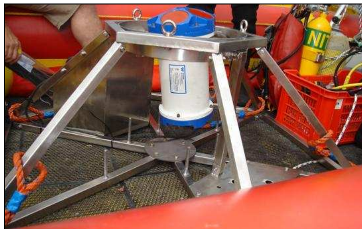
Figure 2 – ADCP frame with 600KHz instrument.
