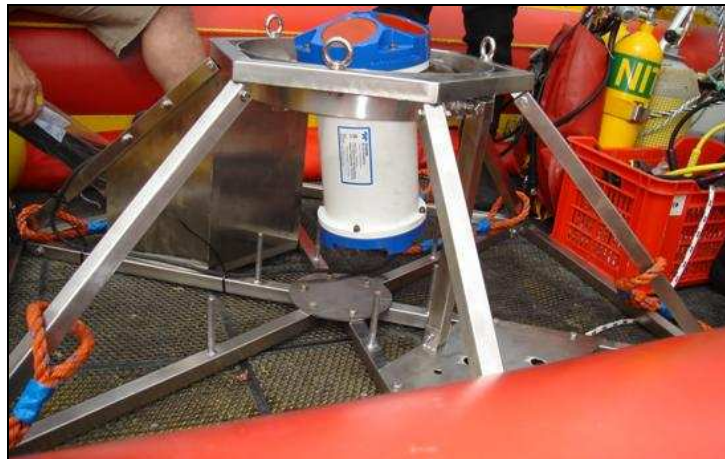
Figure 4 – ADCP frame with 600KHz instrument.
