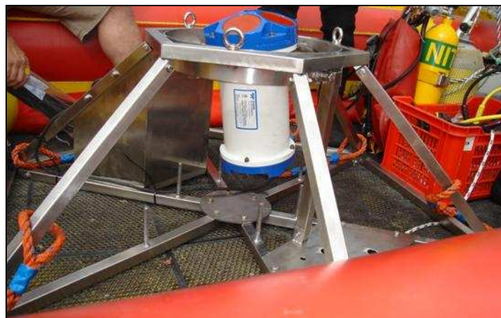
Figure 2 – ADCP frame with 600KHz instrument.
