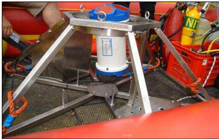
Figure 2 – ADCP frame with 600KHz instrument.
