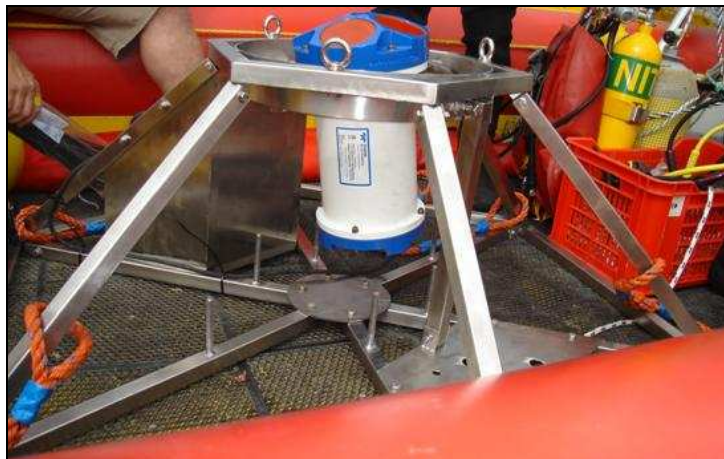
Figure 2 – ADCP frame with 600KHz instrument.
