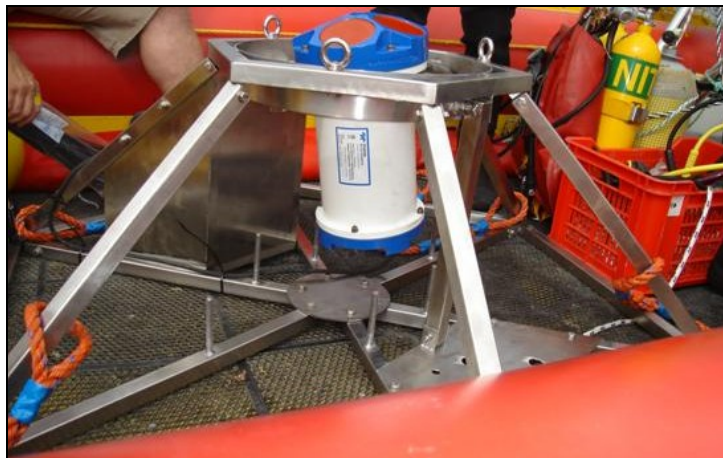
Figure 2 – ADCP frame with 600KHz instrument.
