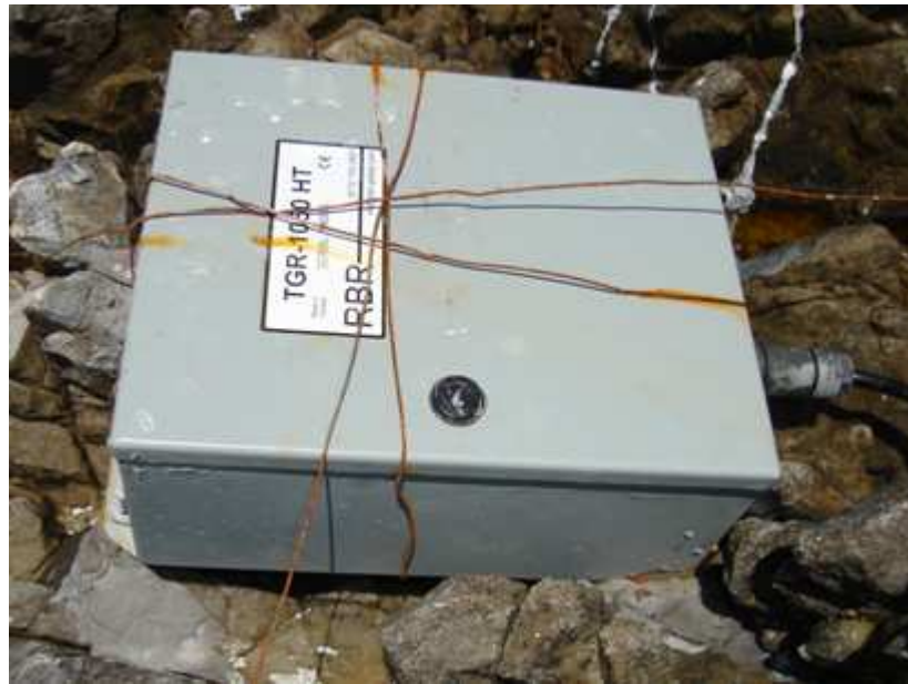
Figure 3- The tide gauge's logger box
