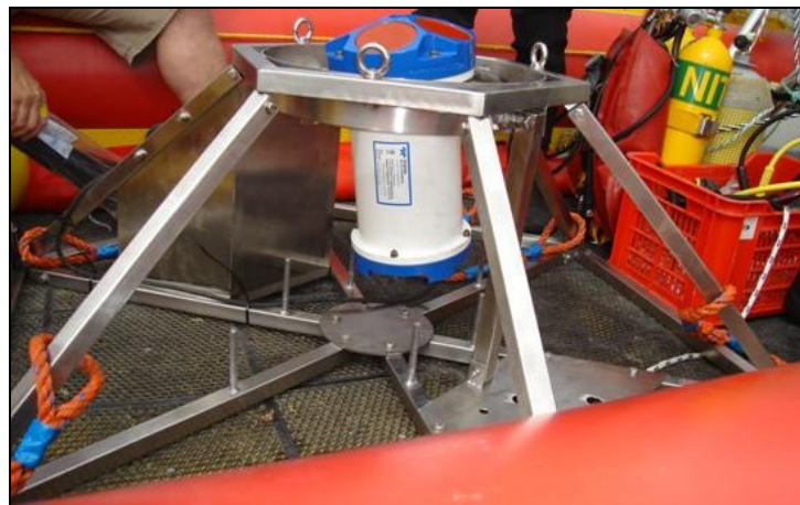
Figure 2 – ADCP frame with 600KHz instrument.
