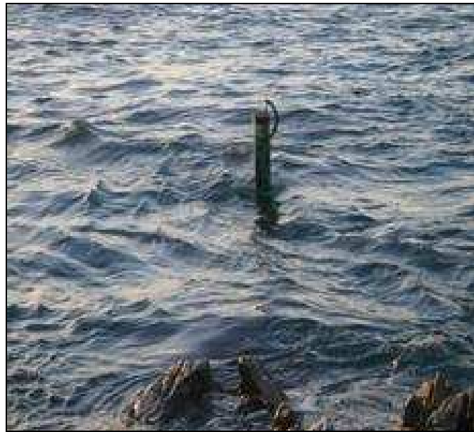
Figure 5-Stilling well protruding from the surface
