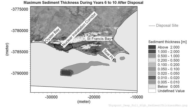
Figure C3: Thyspunt: Maximum sediment thickness for Marine Disposal Alternative 4 (deep disposal site, full sediment volume, high discharge rate)
