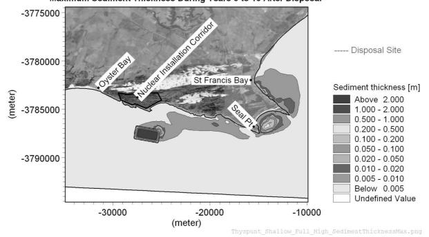
Figure C2: Thyspunt: Maximum sediment thickness for Marine Disposal Alternative 1 (shallow disposal site, full sediment volume, high discharge rate)
