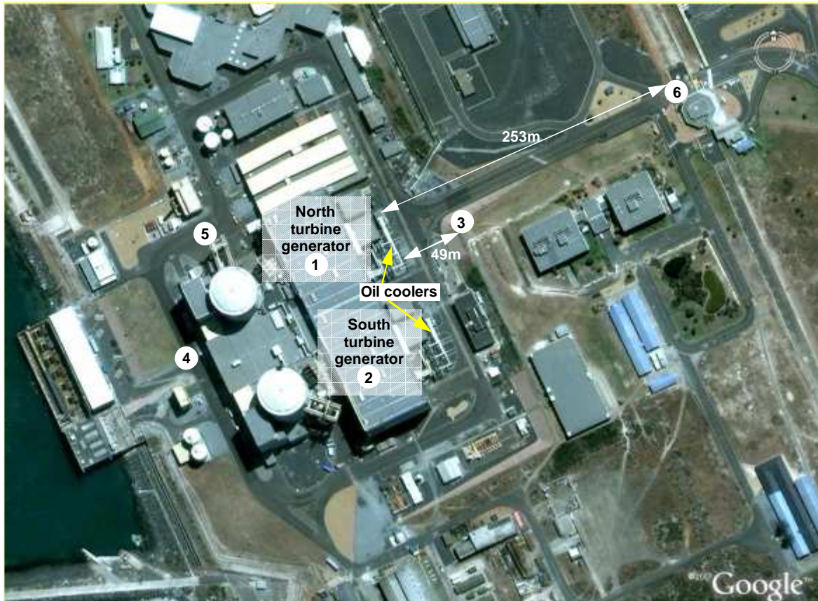
FIGURE 5 Aerial photograph of Koeberg Nuclear Power Station indicating sound measurement locations. Reference: Google Earth
