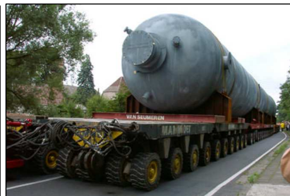
Figure 7.15: SPMT utilising the entire width of road
