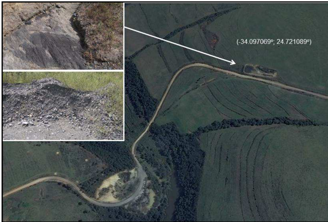
Figure 4-11: Thyspunt – Quarry where shale aggregate is sourced, also showing the material when in-situ
