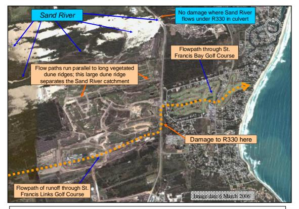
Figure 4.1. Flow path of floodwater that damaged the R330 on 23-24 November 2007. The map is in three parts, top to bottom is from west to east.
