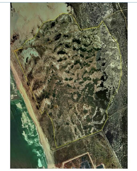
Figure 23. Transverse dune system just north of the existing Koeberg Power Station and actively planted with marram grass between 1979 and 1983. Supplied by Mr Gert Greeff of Eskom
