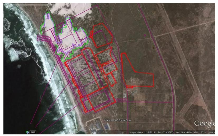
Figure 24. Google image (17 January 2015) showing Koeberg Power Station in the south, with the transverse dunes to the north. The proposed new Nuclear Power Station footprint (red) lies over vegetated transverse dunes. It is this area which was actively stabilised between 1979 and 1983. Shrinkage of the mobile dunes is shown by comparing the edge of bare sand between 2003 (green) and 2014 (mauve). Initial footprint (purple) shown for comparison (see Figure 5.1.2 in botanical EIA)
