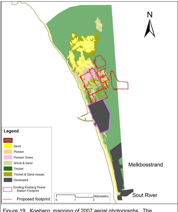
Figure 19. Koeberg: mapping of 2007 aerial photographs. The transverse dunes north of the Power Station continue to show an increase in vegetation cover, with both the pioneer, and thicket and sand mosaic forms dominating. Dune mobility is now severely reduced and is some distance from the Power Station. Thicket, probably mostly acacias, continues to dominate. Development marked in the south
