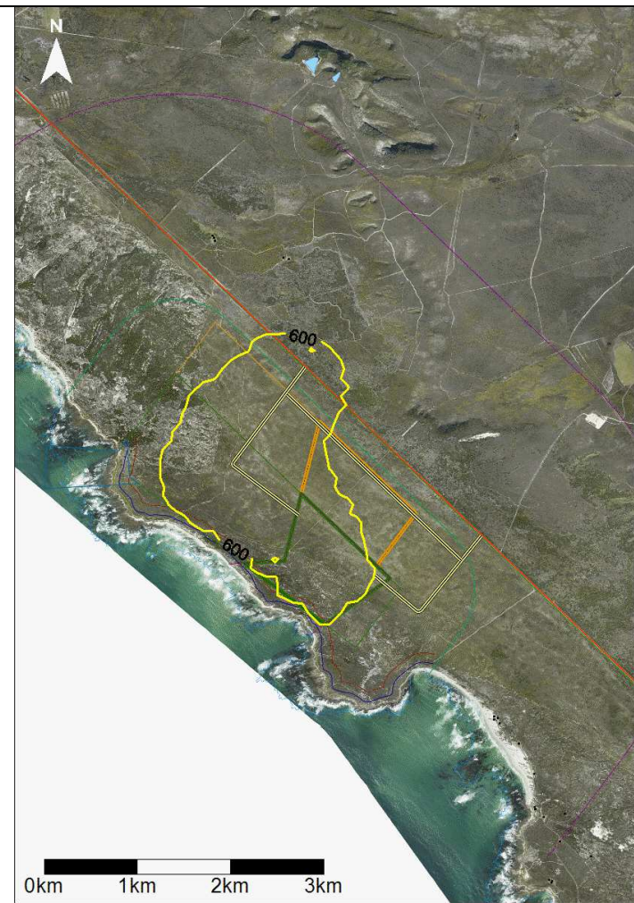
Figure 1-10: Predicted maximum daily average particle fallout rates ( \text{mg}/\text{m}^2/\text{day} ) during construction at Bantamsklip (Unmitigated)
