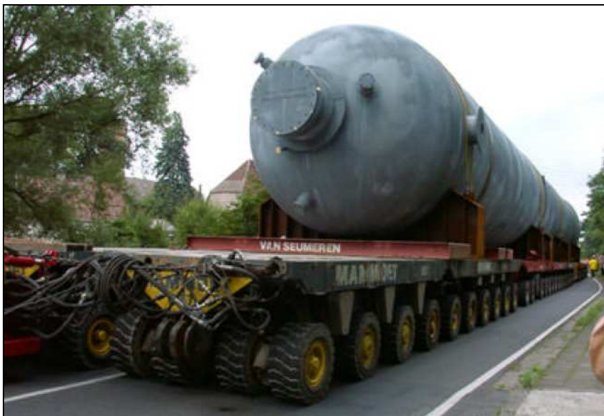
Figure 1-29: A SPMT utilising the entire width of a road
