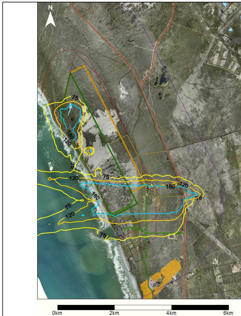
Figure 1-7: Predicted maximum daily average inhalable particle (PM10) concentration levels ( \mu\text{g}/\text{m}^3 ) during construction at Dufnefontein (Unmitigated)
