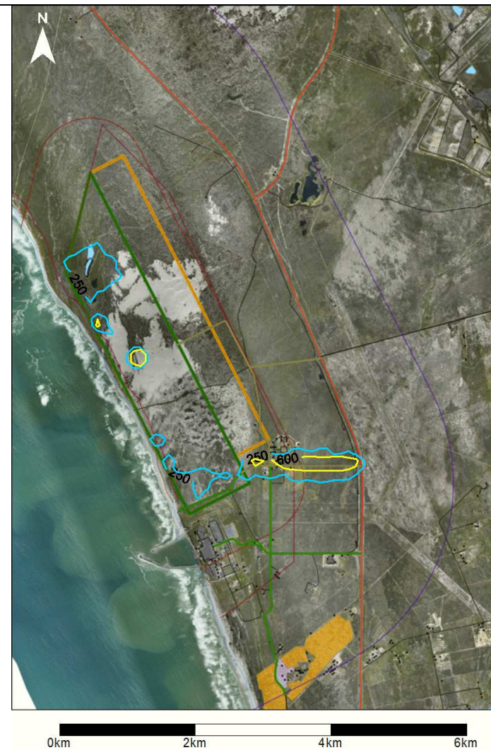
Figure 1-8: Predicted maximum daily average particle fallout rates ( \text{mg}/\text{m}^2/\text{day} ) during construction at Dufnefontein (Unmitigated)
