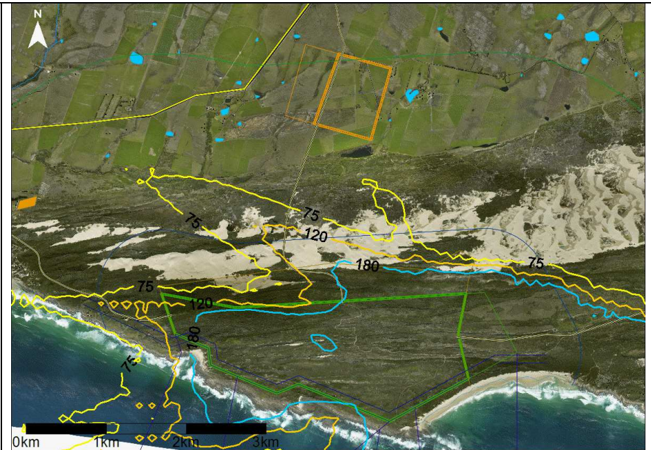
Figure 1-14: Predicted maximum daily average PM10 concentration levels during construction at Thyspunt with Road Option C and the envelope of the nuclear power station on the east or west of the corridor (Unmitigated)
