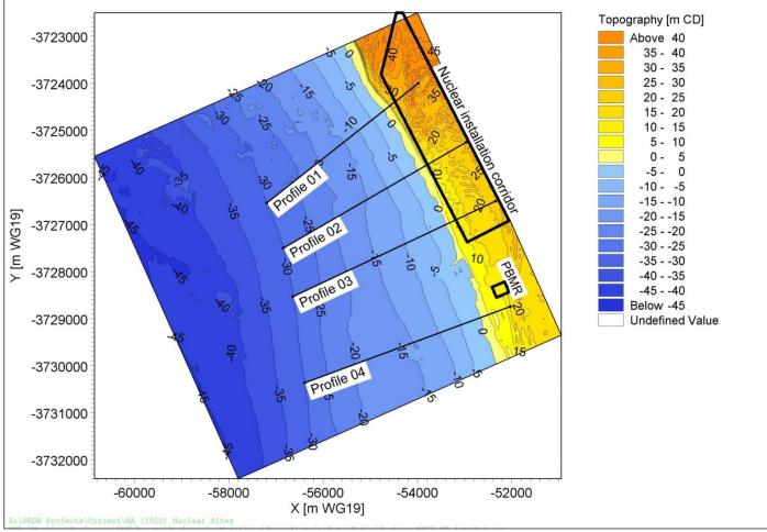
Figure 9-5: Profile locations and bathymetry for Duynefontein
