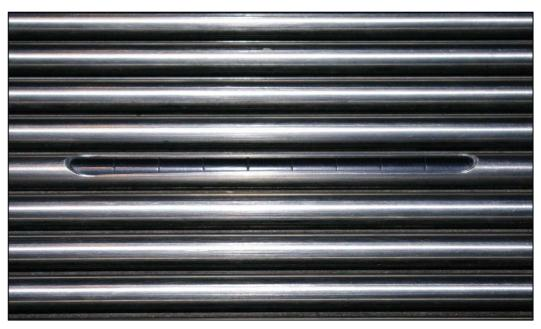
Figure 3-4: A display of nuclear fuel pellets in a cladding tube at Koeberg Nuclear Power Station
