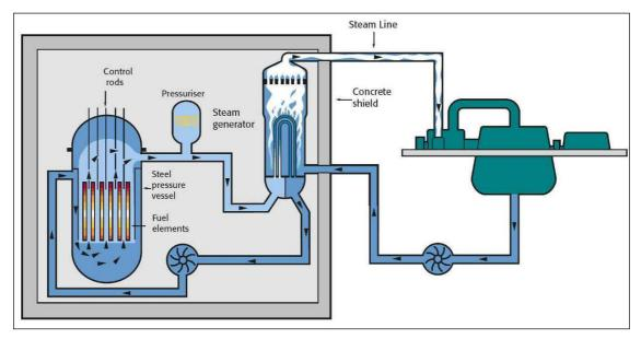
Figure 3-2: Simplified diagrammatic depiction of a Pressurised Water Reactor (PWR)<sup>6</sup> (Ragheb, 2008)
