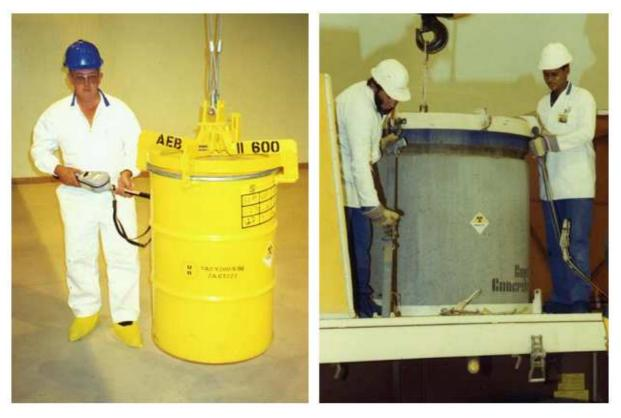
Figure 3-13: Standard steel and concrete containers used for radioactive waste disposal at Vaalputs
