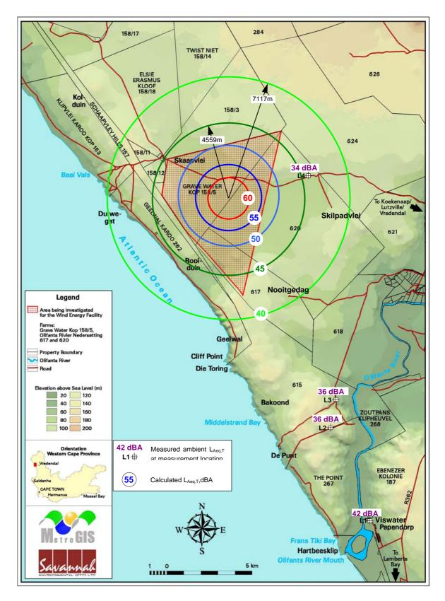
FIGURE 2 Map of study area including ambient sound measurement locations with measured  $L_{Aeq,T}$  and approximate contours of predicted  $L_{Aeq,T}$  emanating from 100 Vestas V66 turbines located at the central area of the proposed site.
