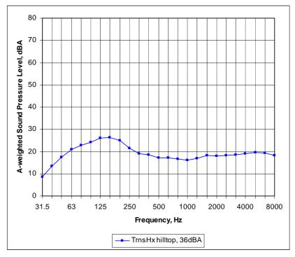
FIGURE 6 Sound level spectrum measured at location L2
