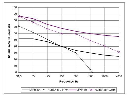
FIGURE 11 Low Frequency Noise Rating curves superimposed onto calculated outdoor octave band sound pressure levels
