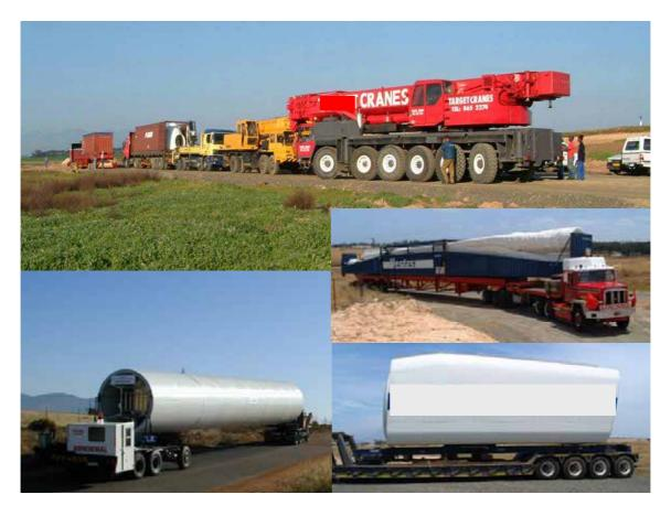
Figure 7.5: Photograph illustrating the equipment required for the transportation of turbine components to site (photographs courtesy of Eskom at during the construction of the Klipheuwel demonstration facility)
