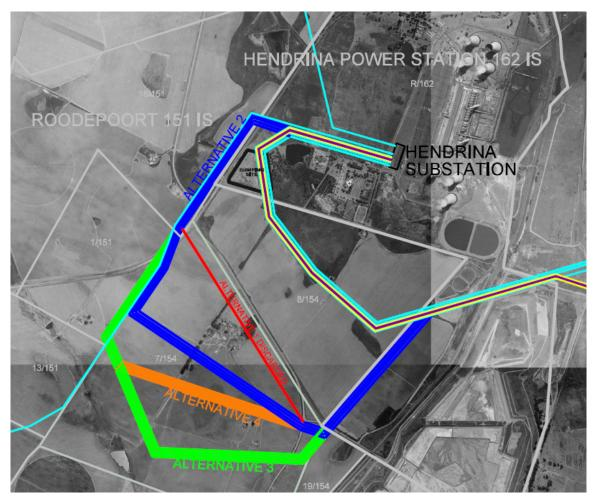
Figure 2. Proposed corridor alternatives for the four 132kv powerlines
