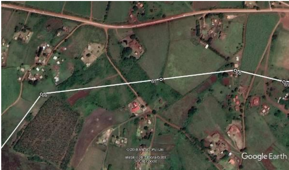
Fig. 24 Bush to be cleared between tower 67 and 68
