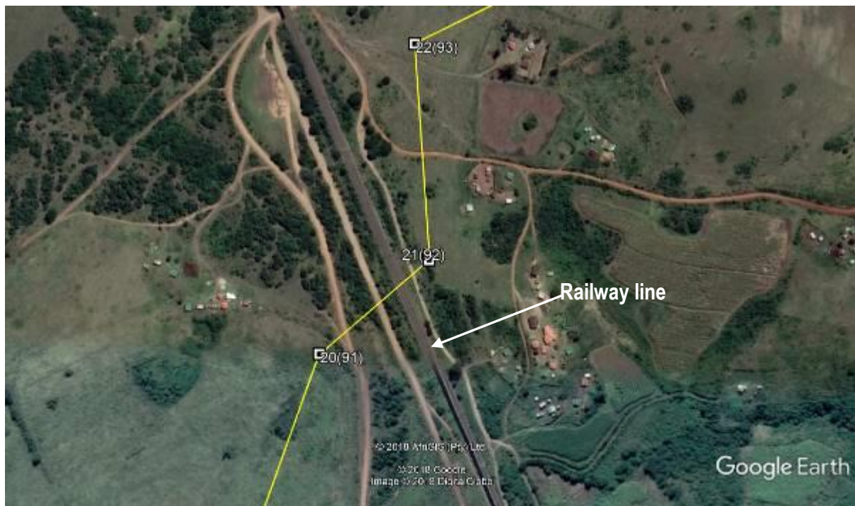
Fig. 29 Showing span between towers 20(91) and 21(92) over a railway line
