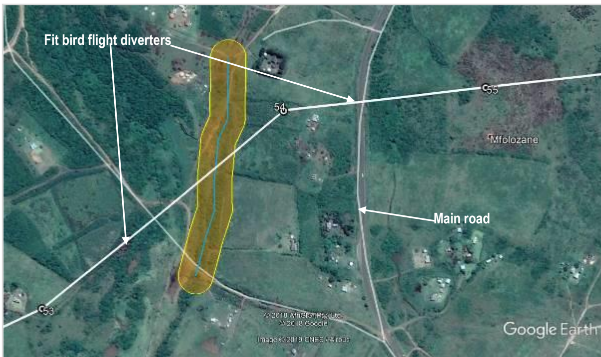
Fig 34 Showing spans requiring bird flight diverters
