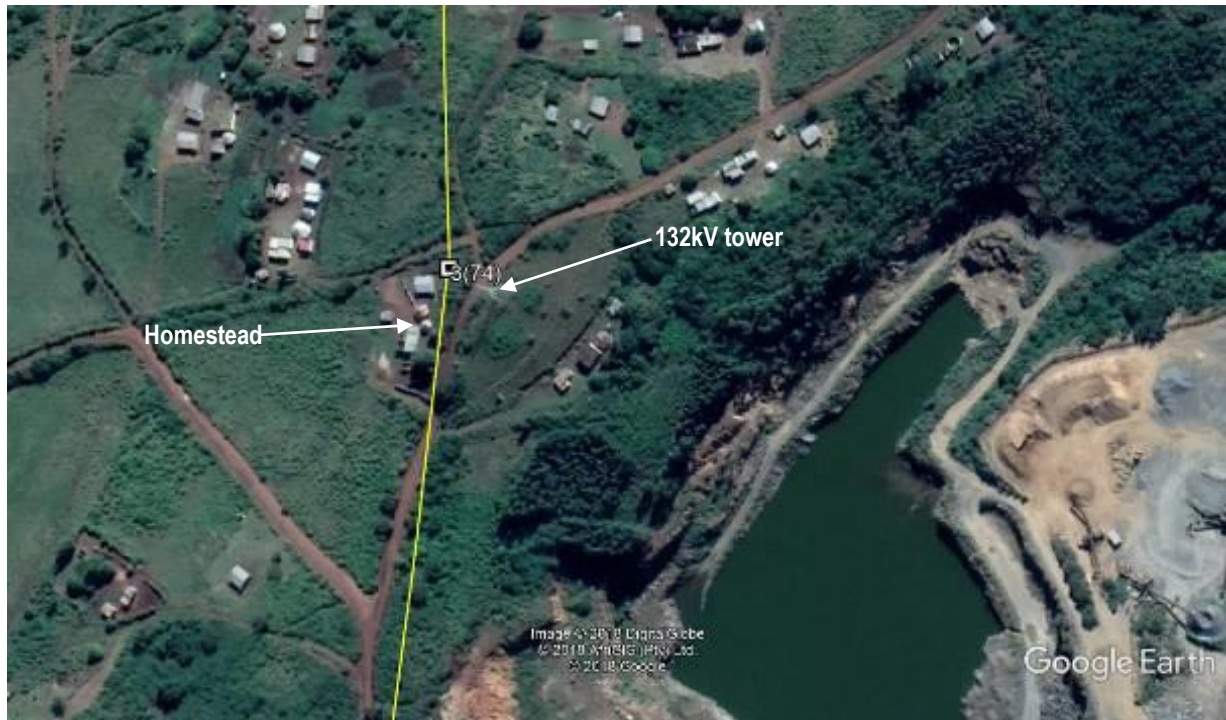
Fig. 26 Shows servitude over a homestead near tower 3(74)
