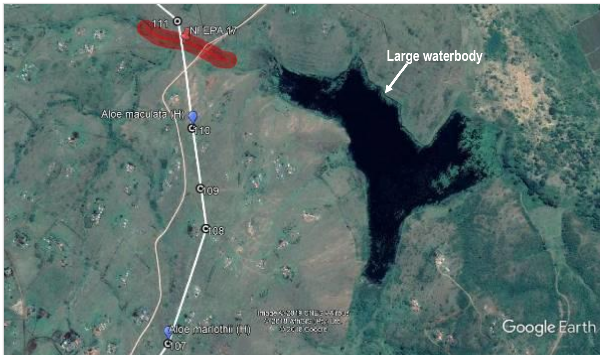
Fig 46 Showing NFEPA wetland and a large waterbody and spans from towers 107(178) – tower 111(182) requiring bird flight diverters
