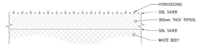
Figure 33. Proposed capping of the ADF.
