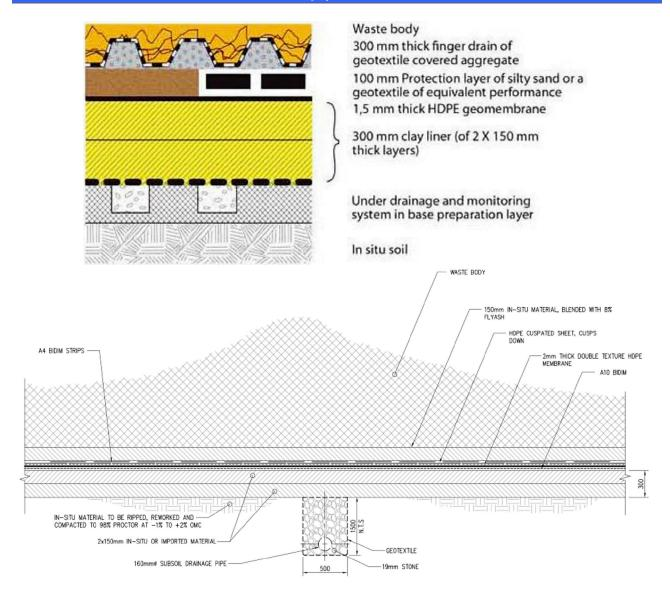
Figure 32. Diagrams showing a typical class C liner and the proposed lining and subsoil drain system for the Kendal 30-year ADF.
