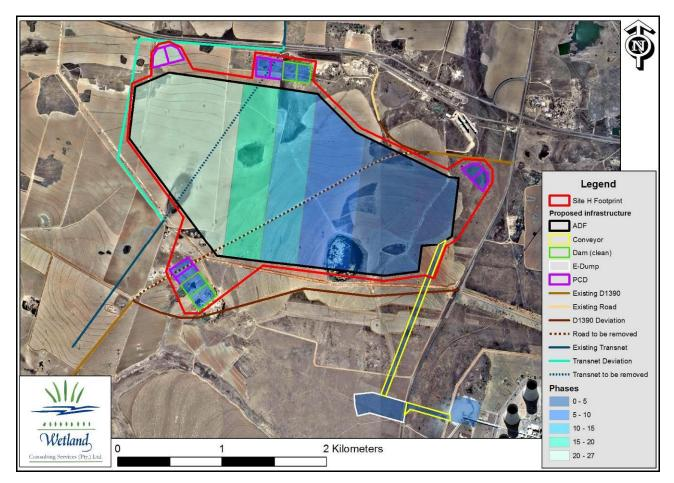
Figure 31. Map showing the proposed footprint of the ADF indicating position of PCD's and the phased nature of development.
