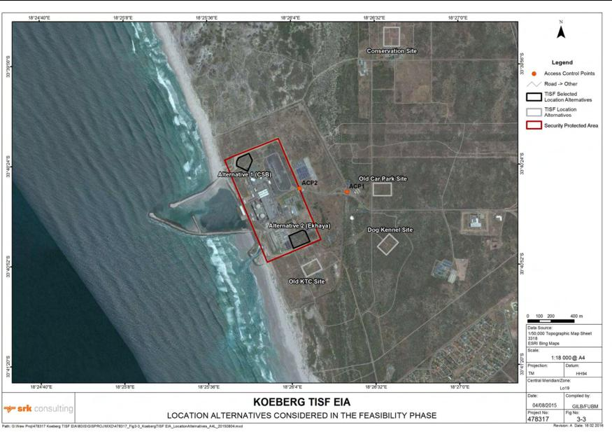
The site selection process eliminated four sites and identified two viable site locations for the TISF i.e. the CSB site - the preferred alternative (Alternative 1) - and the Ekhaya site (Alternative 2) (Figure 3-3). Alternative 1 is located adjacent to the CSB on the northern boundary of KNPS and Alternative 2 is located along the southern boundary of KNPS next to the Ekhaya Building.
