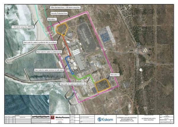
Figure 3-5: Transfer routes from the SFP to the TISF (Alternative 1 and 2) *Source: Eskom, 2016*
