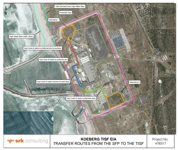
Figure 3-5: Transfer routes from the SFP to the TISF (Alternative 1 and 2)
