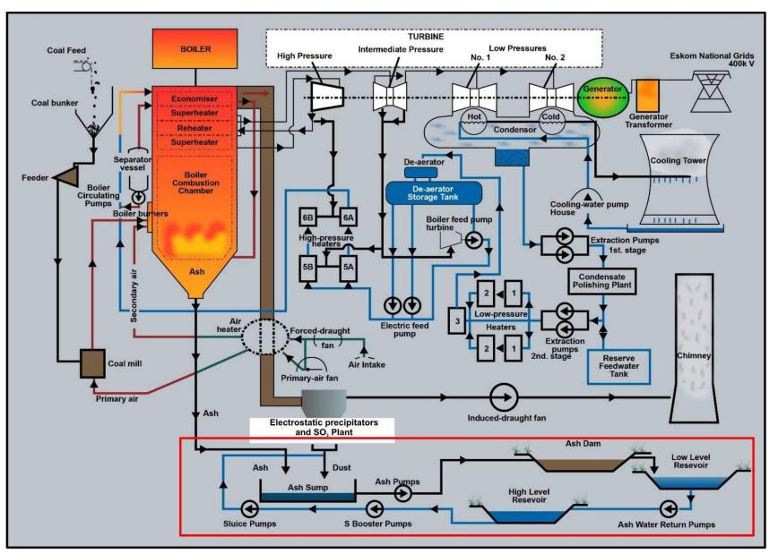
Figure 2: Flowchart of the operation, showing inputs and outputs of the process (including the Ash Disposal Facility in red)
