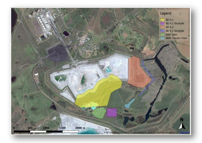
Figure 2: Aerial image zoomed in showing the position of the proposed ash dams, return water dams and stockpile areas
