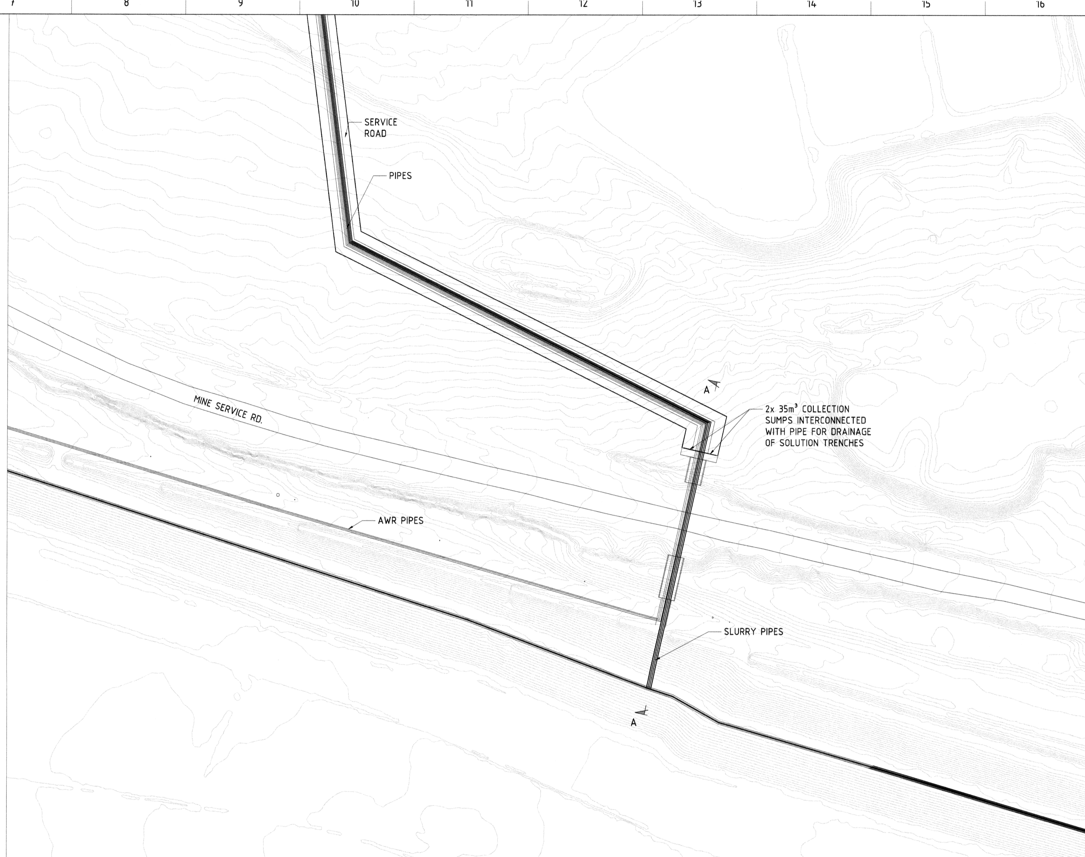
PLAN SHOWING PIPE CROSSING
