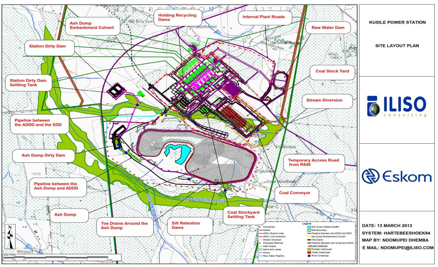
Figure 1-0-1: Kusile Site Layout Plan showing the River and Wetland Crossings being Applied For
