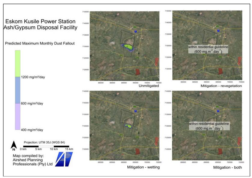
Figure 5-1: Predicted maximum monthly dust deposition as a result of windblown dust from the disposal facility at the Kusile Power Station
