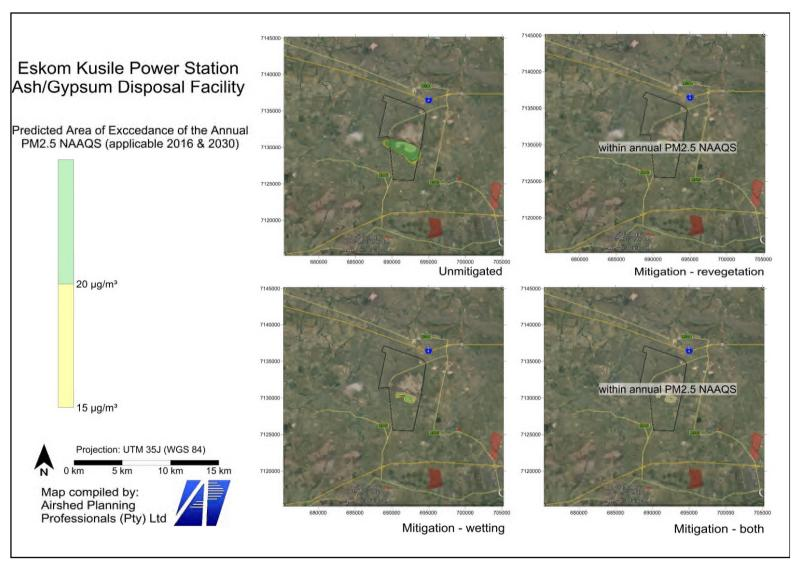
Figure 5-5: Predicted annual average PM<sub>2.5</sub> concentrations due to the disposal facility at Kusile Power Station
