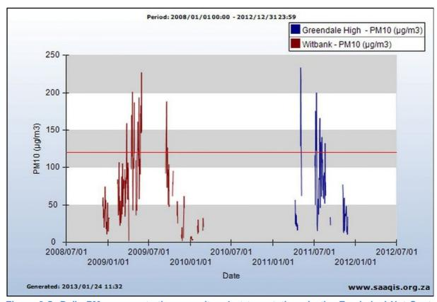
Figure 3-5: Daily PM<sub>10</sub> concentrations monitored at two stations in the Emahaleni Hot Spot between 2008 and 2012 (from <u>www.saaqis.org.za</u>). The horizontal red line indicates the current daily limit of 120 μg.m<sup>-3</sup>.
