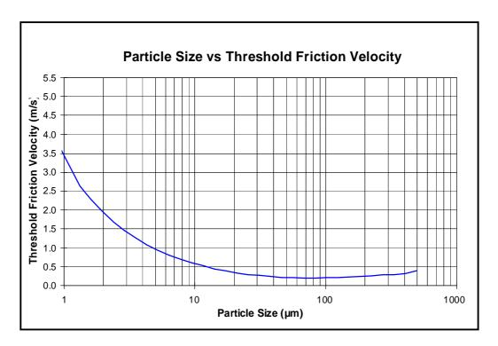
Figure A-1: Relationship between particle sizes and threshold friction velocities using the calculation method proposed by Marticorena and Bergametti (1995)
