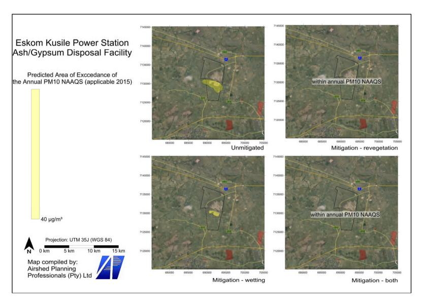
Figure 5-3: Predicted annual average PM<sub>10</sub> concentrations due to the disposal facility at Kusile Power Station
