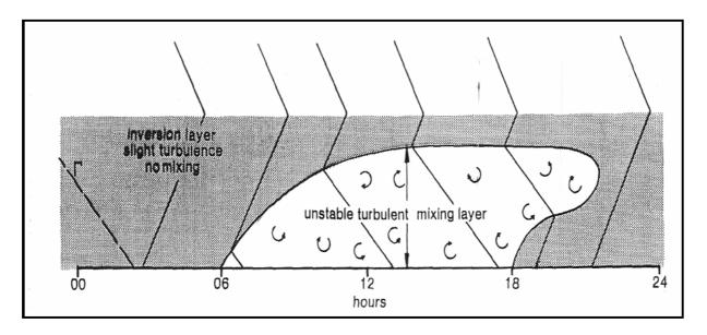
Figure 3-4: Daytime development of a turbulent mixing layer (Preston-Whyte & Tyson, 1988)
