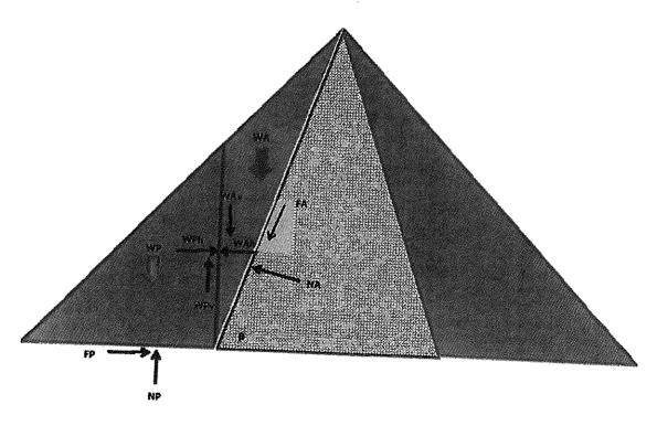
Since the concrete is a stiff member with low strain compared to either the coal, the HPDE/GCL liner of the foundation, the fully developed lateral force results in tension forces in the concrete, without shedding load via shear to the substrate. These tension forces were determined using both translational failure (shown above) and finite element analyses. The maximum tensile force in the reinforced concrete liner is 510kN/m for the given coal geometric criteria
