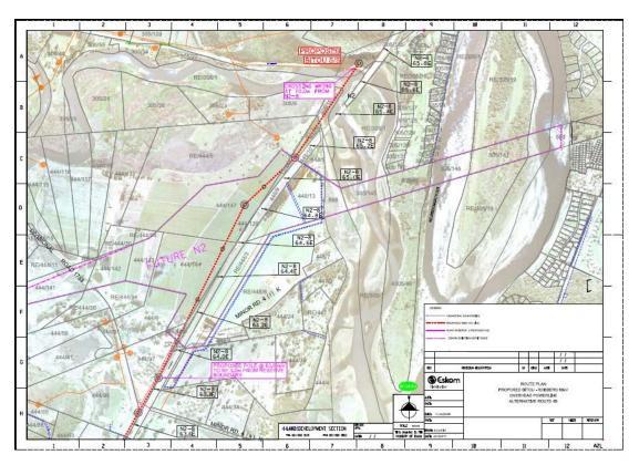
Figure 1. Site plan showing the direction of the proposed power line route (dotted red line) and supporting pylons.
